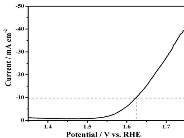
**Figure S9** Polarization curve of CoMoO<sub>4</sub> powder sample on a 3 mm glassy carbon electrode.
