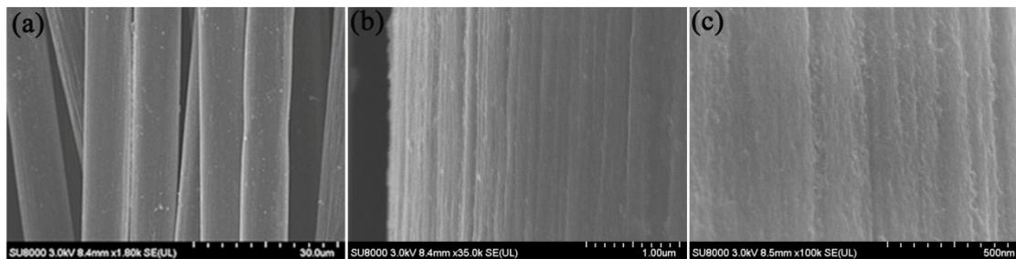
**Figure S2** Low- and high-magnification SEM images of bare carbon cloth.
