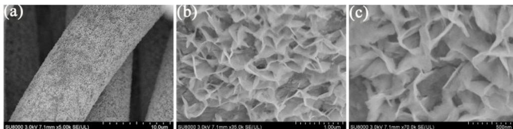
**Figure S10** Low- and high-magnification SEM images of  $\text{CoMoO}_4\text{-CC}$  after stability tests.
