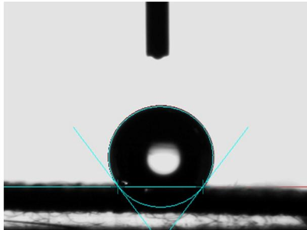
**Figure S1** Contact angle measurement on the electrode of bare carbon cloth.
