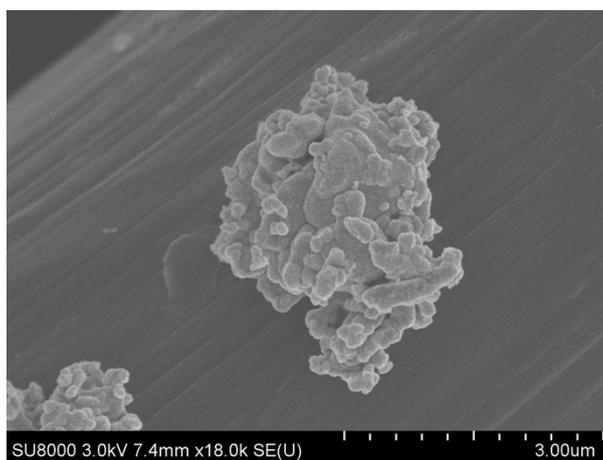
**Figure S6** SEM image IrO<sub>2</sub>-CC<sup>a</sup>.
