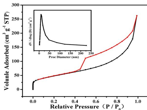
**Figure S7** Nitrogen adsorption–desorption isotherms of as-synthesized NiMoO<sub>4</sub> nanosheets scratched from the carbon fiber.
