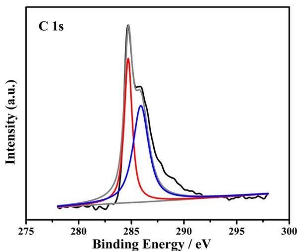
**Figure S8** C<sub>1s</sub> core-level XPS of CoMoO<sub>4</sub>-CC.
