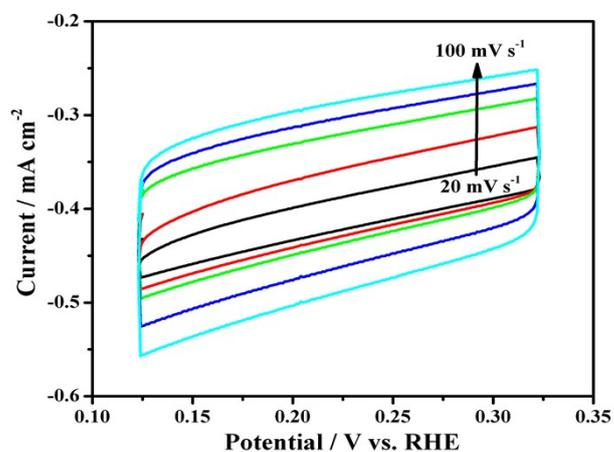
**Figure S11** Electrochemical cyclic voltammetry curves of  $\text{NiMoO}_4\text{-CC}$  at different potential scanning rates. The selected potential range is 0.12 - 0.32 V vs. RHE where no faradic current was observed.
