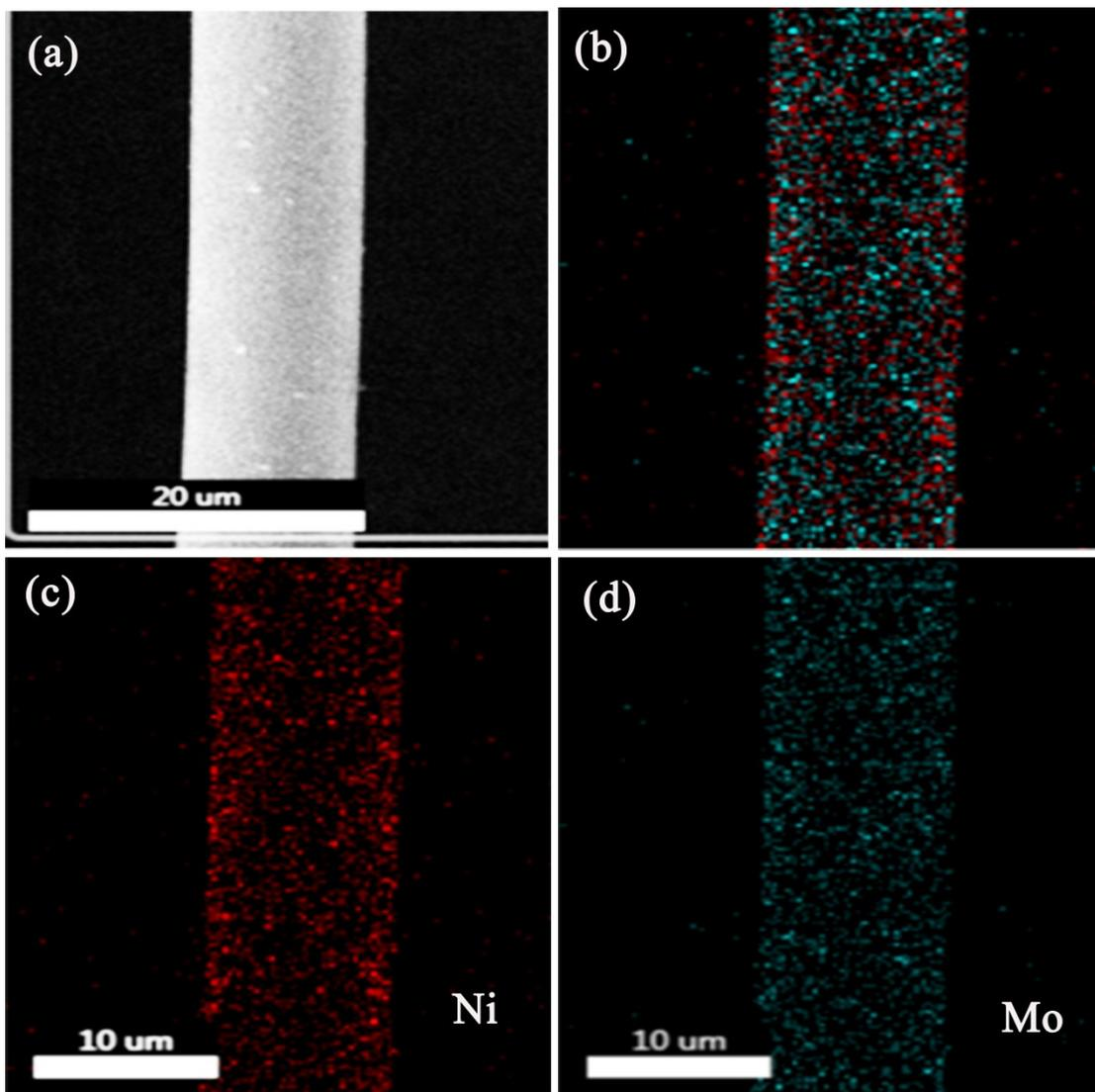
**Figure S5** SEM-EDX elemental maps of Mo and Ni for NiMoO<sub>4</sub>-CC.
