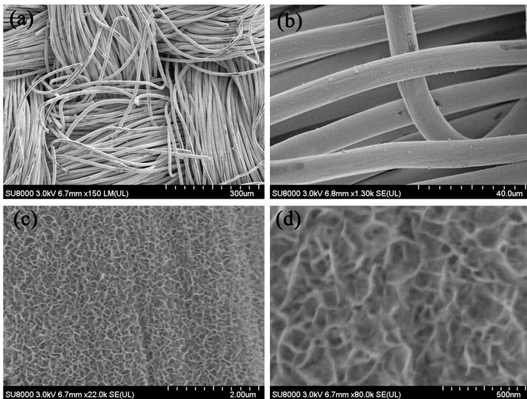
**Figure S4** Low- and high-magnification SEM images of NiMoO<sub>4</sub>-CC.
