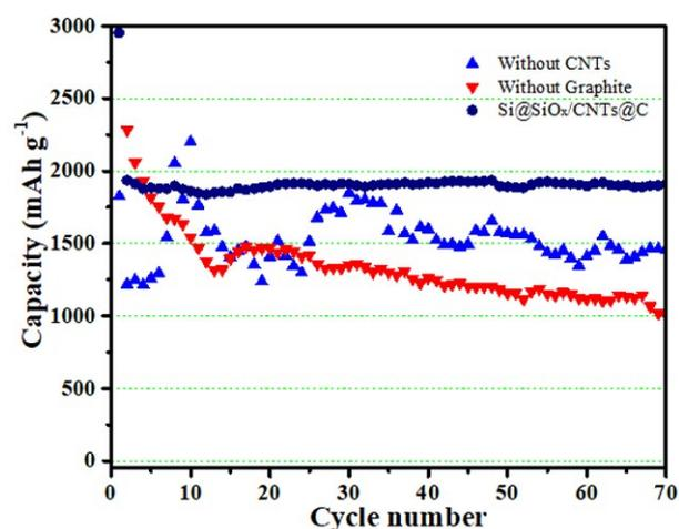
Fig. S2. Cycling performance of composite material with various component combinations at current density of 0.42 A g<sup>-1</sup>.
