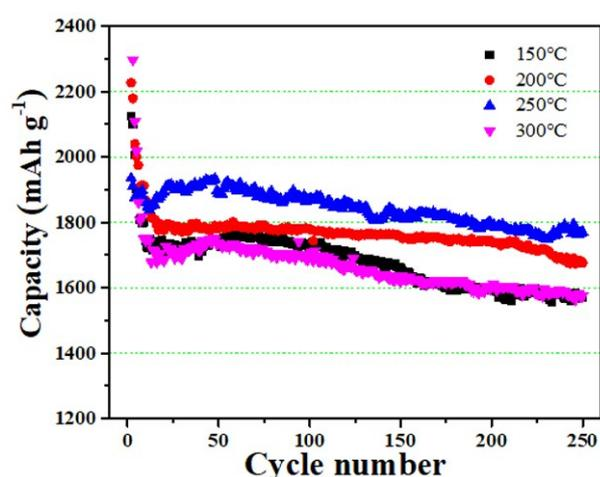
Fig. S1. Cycling performance of composite material with different oxidation temperatures at current density of 0.42 A g<sup>-1</sup>
