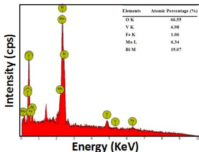
**Fig. S3** EDS pattern of the as-prepared Fe/Mo-BVO PNSs and the atom percentages of O, V, Fe, MO and Bi elements (inset).
