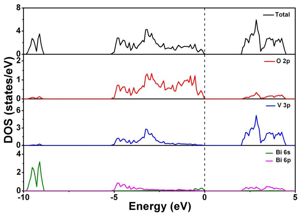
**Fig. S5** Total DOS and the corresponding PDOSs of O2p, V3p, Bi 6s and Bi 6p states of pure BVO.
