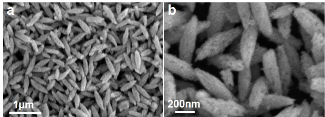
**Fig. S7** SEM images of the as-prepared Fe/Mo-BVO PNSs after photocatalytic water oxidation test under visible-light irradiation.
