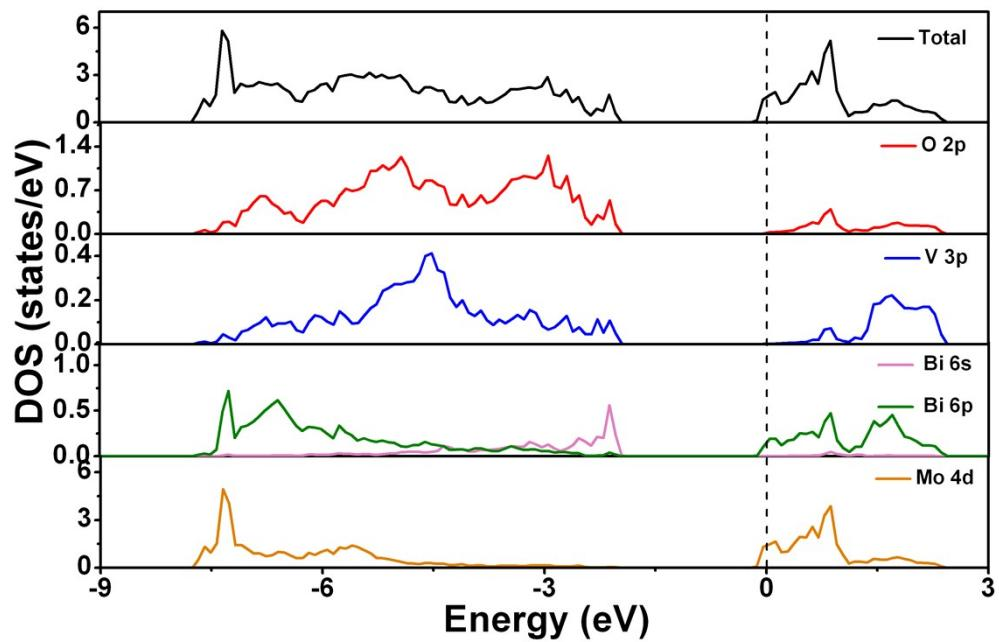
**Fig. S6** Total DOS and the corresponding PDOSs of O<sub>2</sub>p, V3p, Bi 6s, Bi 6p, and Mo 4d states of Mo-BVO.
