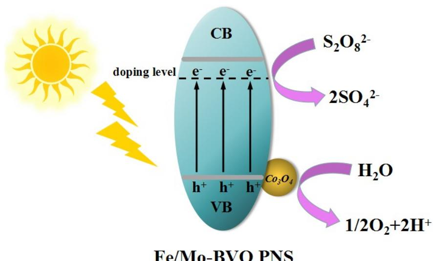
**Scheme S1** Schematic illustrating the mechanism of the as-prepared Fe/Mo-BVO PNS for water oxidation under visible-light irradiation.
