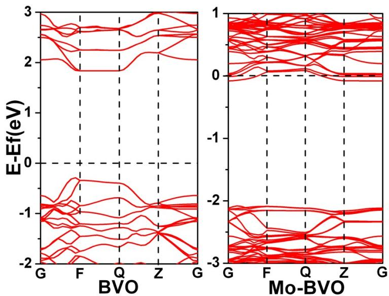
**Fig. S4** The band structures calculated for the BVO and Mo-BVO crystal structures.
