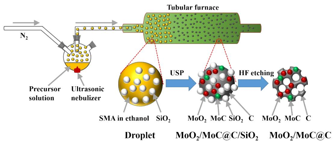
**Fig. S1.** The setup of synthesis of  $\text{MoO}_2/\text{MoC}@\text{C}$ .
