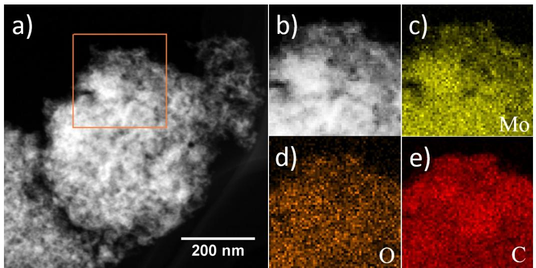
**Fig. S6.** (a, b) STEM images and EDX elemental mapping images of (c) Mo, (d) O, and (e) C elements.
