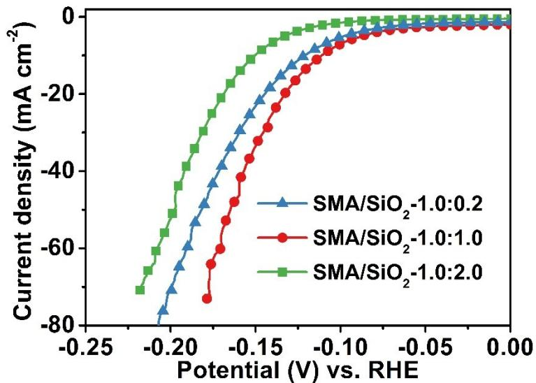
**Fig. S9.** Polarization curves of MoO<sub>2</sub>/MoC@C-850 samples with different ratios of SMA/SiO<sub>2</sub>. For clarification, the as-prepared samples were named SMA/SiO<sub>2</sub>-X, which indicates the mass ratio (X) of SMA to SiO<sub>2</sub> in the synthesis. In the full paper, the samples of SMA/SiO<sub>2</sub>-1.0:1.0 is also named as MoO<sub>2</sub>/MoC@C-850.
