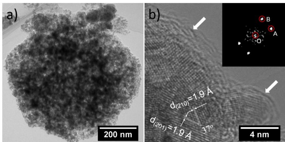
**Fig. S8.** (a) TEM and (b) HRTEM images of  $\text{MoO}_2/\text{MoC}@\text{C}-950$ .
