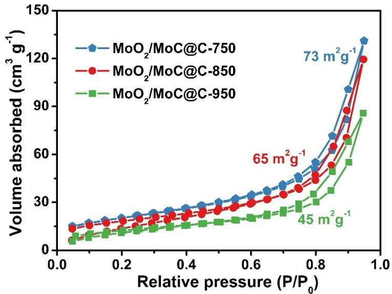
**Fig. S11.** Nitrogen adsorption/desorption isotherm of MoO<sub>2</sub>/MoC@C-750, MoO<sub>2</sub>/MoC@C-850 and MoO<sub>2</sub>/MoC@C-950.
