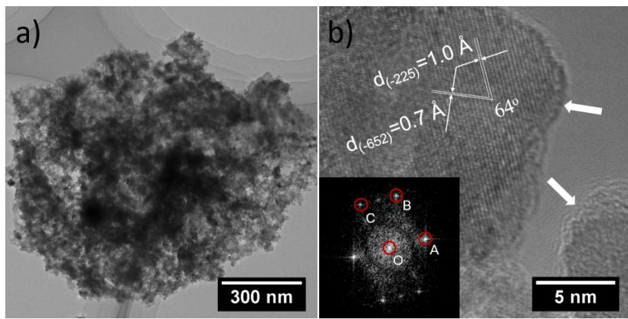
**Fig. S7.** (a) TEM and (b) HRTEM images of  $\text{MoO}_2/\text{MoC}@\text{C}-750$ .
