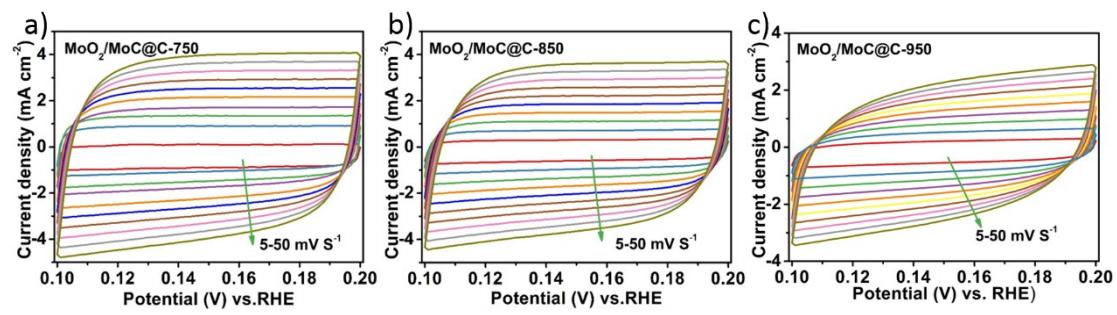
**Fig. S12.** Cyclic voltammograms in the region of 0.1-0.2 V vs. RHE for the (a) MoO<sub>2</sub>/MoC@C-750, (b) MoO<sub>2</sub>/MoC@C-850, and (c) MoO<sub>2</sub>/MoC@C-950.
