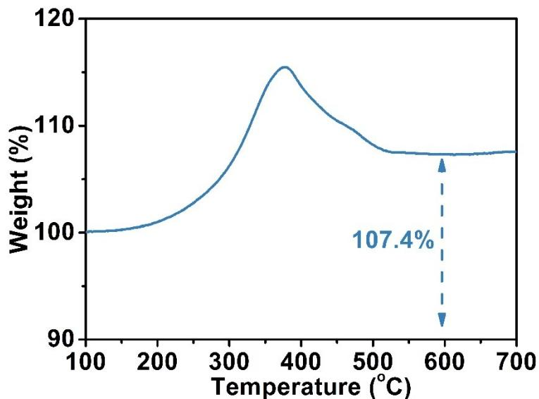
**Fig. S2.** TGA curve of  $\text{MoO}_2/\text{MoC}@\text{C}$  in  $\text{O}_2$  with heating rate of  $10 \text{ }^{\circ}\text{C min}^{-1}$ .
