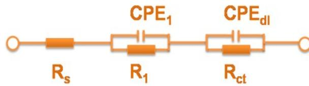
**Fig. S10.** Equivalent circuit used to fit the EIS data.  $R_s$  is the overall series resistance,  $CPE_1$  and  $R_1$  are the constant phase element and resistance describing electron transport at GCE/electrocatalyst interface, respectively,  $CPE_{dl}$  is the constant phase element of the electrocatalyst/electrolyte interface, and  $R_{ct}$  is the charge transfer resistance at electrocatalyst /electrolyte interface.
