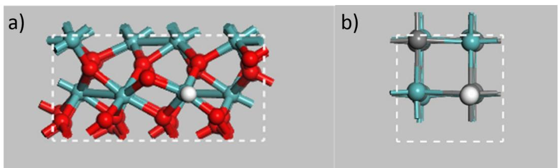
**Fig. S13.** Optimized structures of H\* adsorbed on the surface of (a) MoO<sub>2</sub> (101) plane and (b) MoC (001) plane. Cyan balls denote molybdenum atoms, red ones denote oxygen atoms, gray ones denote carbon atoms, and white ones denote hydrogen atoms.
