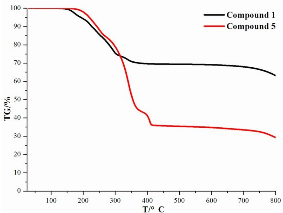
**Fig. S10 Thermogravimetric curves for 1 and 5**
