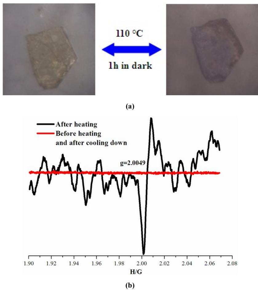
Fig. S6 Thermochromic behavior (a); ESR spectrum of before/after heating and after cooling down in 2 (b)
