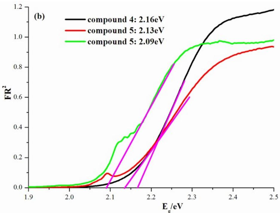
Fig. S5 Diffuse reflectance spectra of 1-3 (a) and 4-6 (b) in Kubelka-Munk unit
