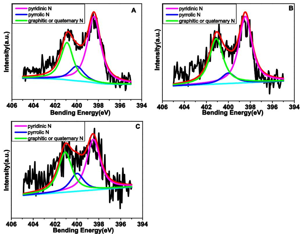
Figure S28. N 1s XPS spectrum of NZ<sub>x</sub>-C, A) NZ<sub>0.5</sub>-C, B) NZ<sub>1</sub>-C and C) NZ<sub>1.5</sub>-C.
