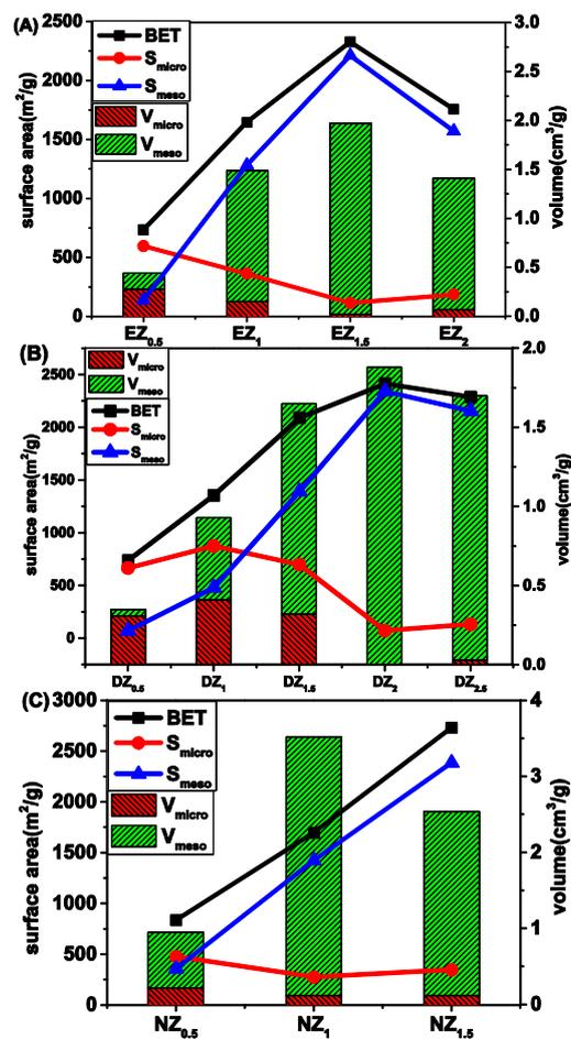
Figure S14. Porous structure parameters of NCFs. EZ<sub>x</sub>-C (A1, A2), DZ<sub>x</sub>-C (B1, B2) and NZ<sub>x</sub>-C (C1, C2).
