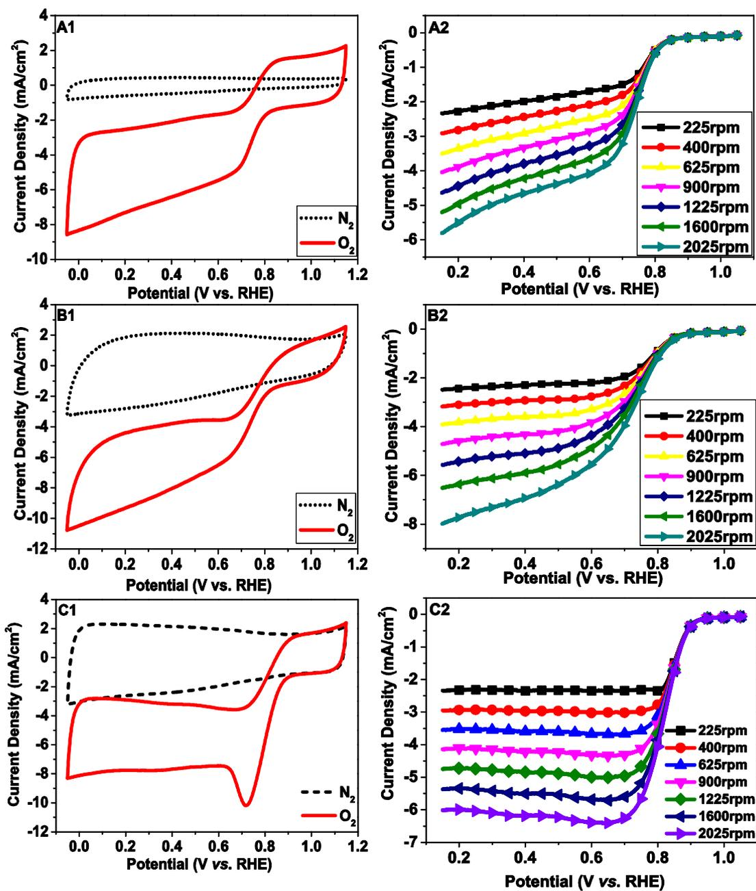
Figure S32. CV and LSV curves of NZ<sub>X</sub>-C, A1, A2 (NZ<sub>0.5</sub>-C), B1, B2 (NZ<sub>1</sub>-C) and C1, C2 (DZ<sub>1.5</sub>-C).
