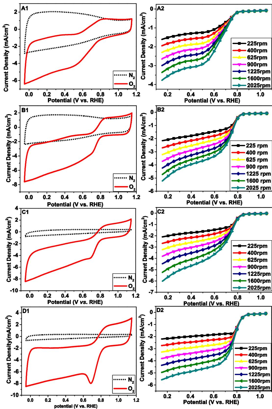
Figure S29. CV and LSV curves of  $EZ_X-C$ , A1, A2 ( $EZ_{0.5}-C$ ), B1, B2 ( $EZ_1-C$ ), C1, C2 ( $EZ_{1.5}-C$ ) and D1, D2 ( $EZ_2-C$ ).
