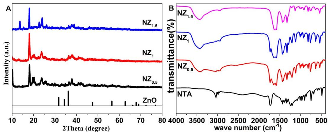
**Figure S6.** XRD (A) and IR (B) curves of  $NZ_x$
