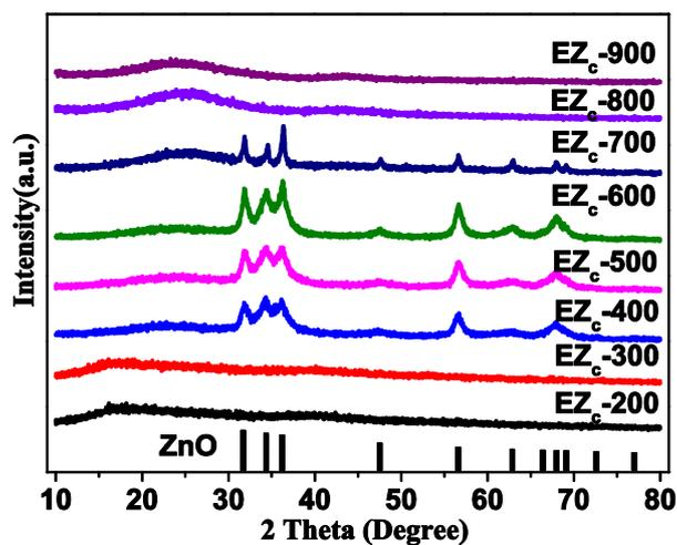
Figure S8. XRD result of EZ1 carbonized at different temperature.
