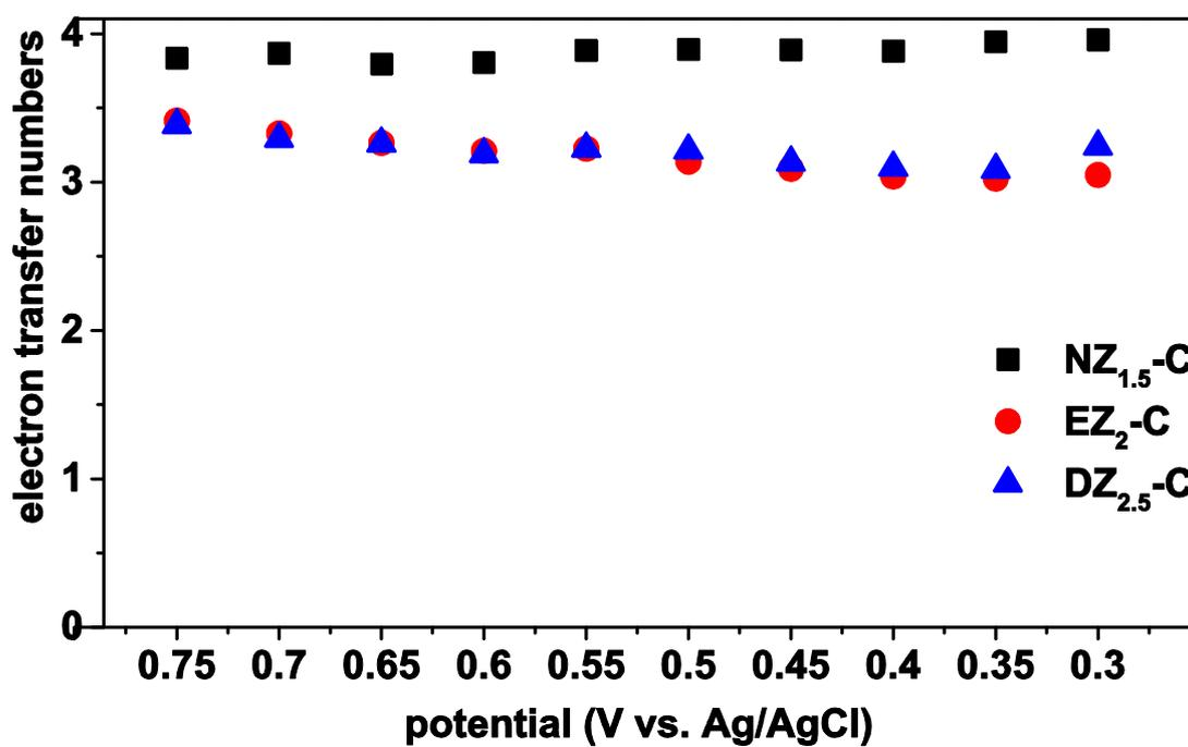
Figure S34. Electron transfer numbers calculated from K-L plots.
