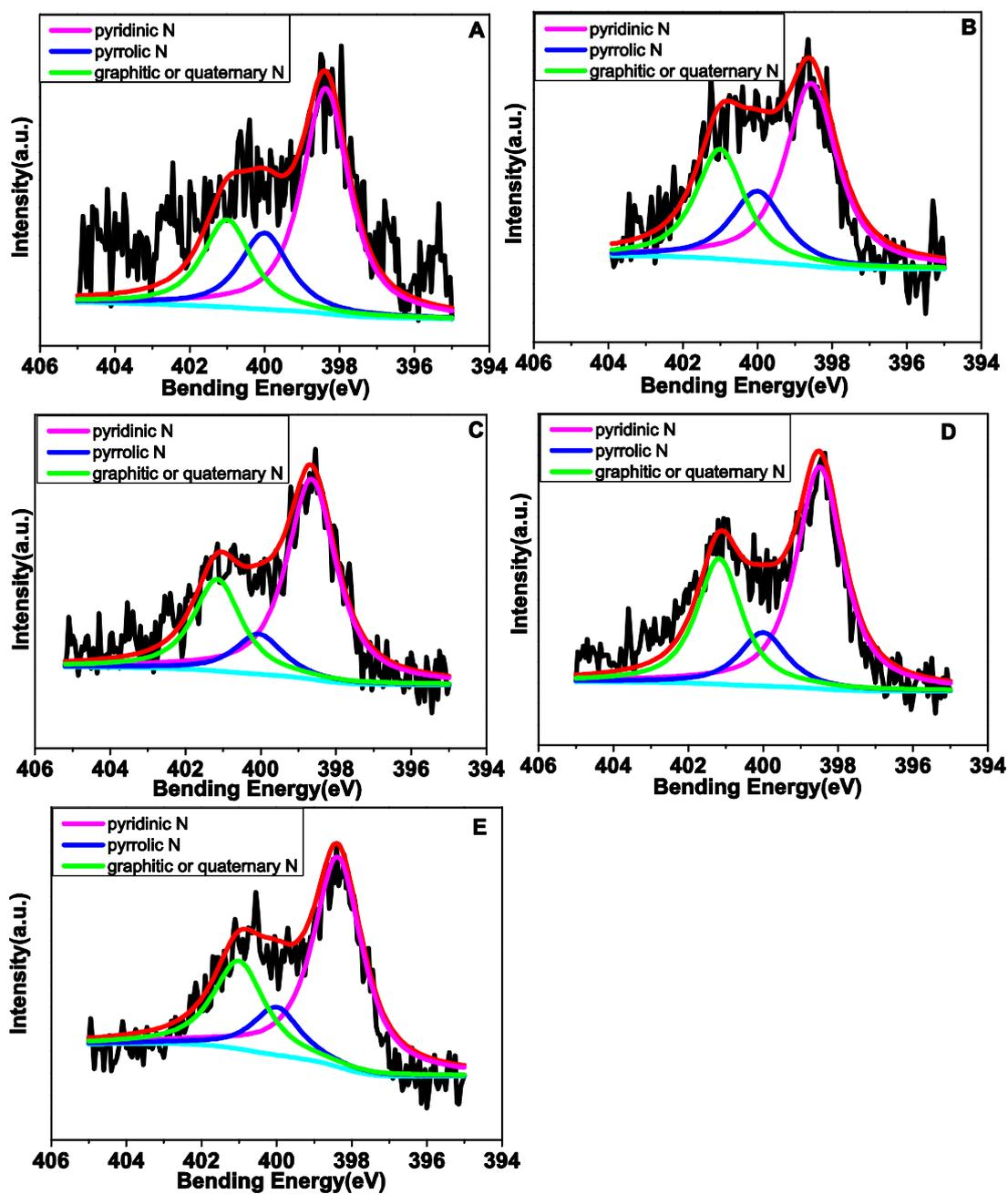
Figure S27. N 1s XPS spectrum of  $DZ_X-C$ , A)  $DZ_{0.5}-C$ , B)  $DZ_1-C$ , C)  $DZ_{1.5}-C$ , D)  $DZ_2-C$  and E)  $DZ_{2.5}-C$ .
