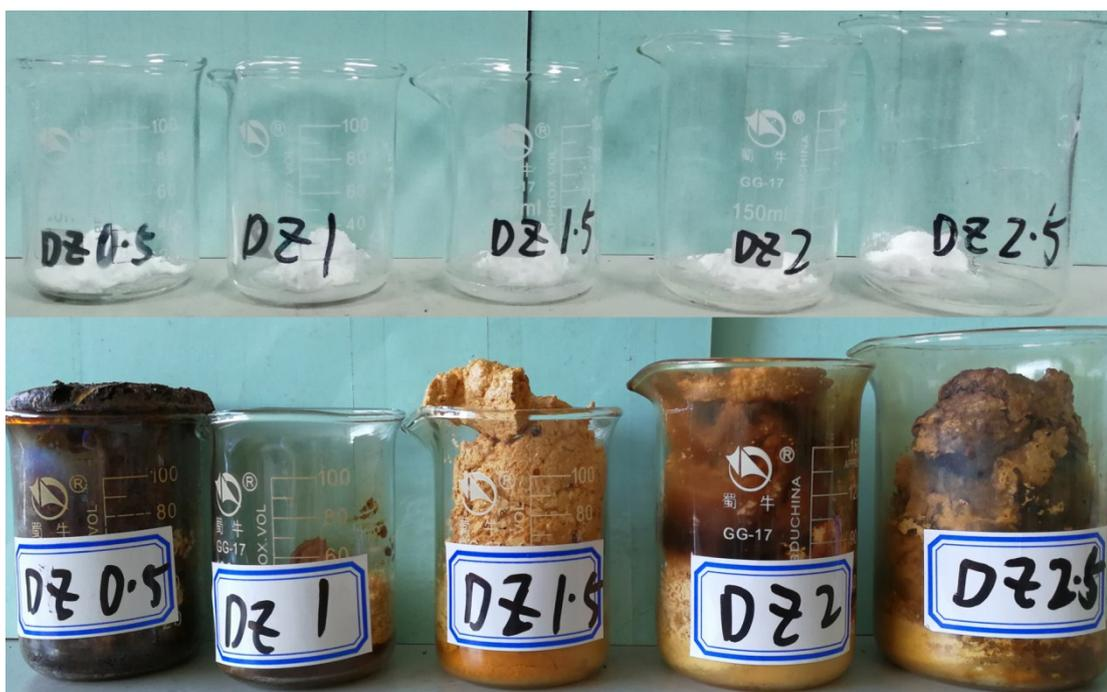
**Fig. S2. Photographs of precursors (up) and 3D Chelates Foams(down) for  $DZ_x$ ,  $DZ_{0.5}$ ,  $DZ_1$ ,  $DZ_{1.5}$  are in 100mL glass beakers.  $DZ_2$  in 100mL glass beaker.  $DZ_{2.5}$  in 200mL glass beaker.**
