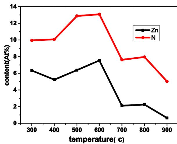
Figure S13. Nitrogen and Zn content for EZ<sub>1</sub>-C from XPS result.
