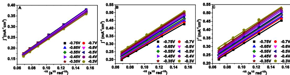
Figure S33. Koutecky-Levich plots at different potentials of A)  $\text{NZ}_{1.5}\text{-C}$ , B)  $\text{EZ}_2\text{-C}$ , C)  $\text{DZ}_{2.5}\text{-C}$ .
