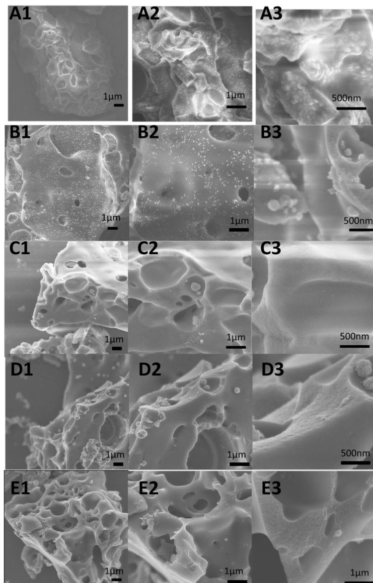
**Figure S10. SEM images of ( A1 - A3 ) EZ<sub>1</sub>-C300, ( B1 - B3 ) EZ<sub>1</sub>-C400, ( C1 - C3 ) EZ<sub>1</sub>-C500, ( D1- D3 ) EZ<sub>1</sub>-C600, ( E1 - E3 ) EZ<sub>1</sub>-C700.**
