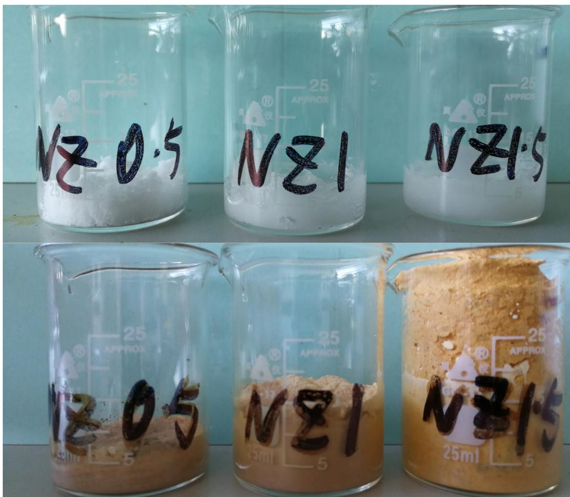
**Fig. S3. Photographs of precursors (up) and 3D Chelates Foams (down) for NZ<sub>x</sub> in 25 mL glass beakers.**
