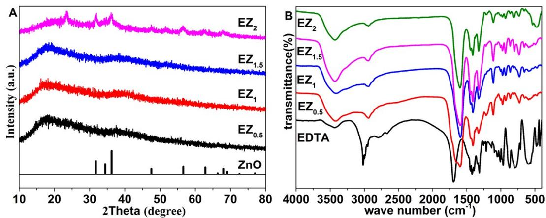
Figure S4. XRD (A) and IR (B) curves of EZ<sub>X</sub>
