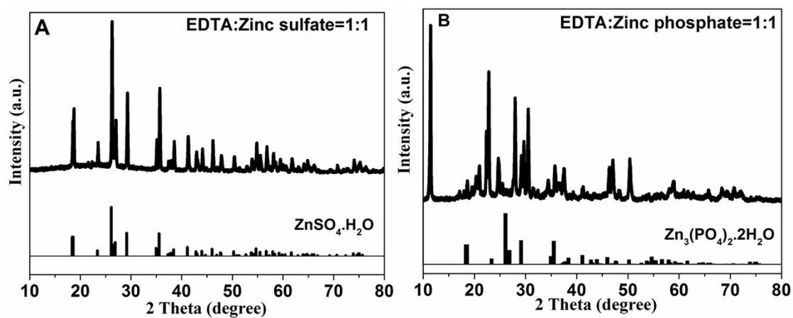
**Figure S7.** XRD results, (A) EDTA heated with Zinc sulfate. (B) EDTA heated with Zinc phosphate.
