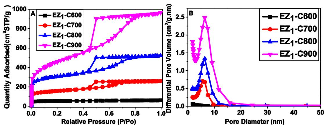
Figure S9. (A) N<sub>2</sub> adsorption isotherms of EZ<sub>1</sub> carbonized at different temperature and (B) corresponding pore size distribution.
