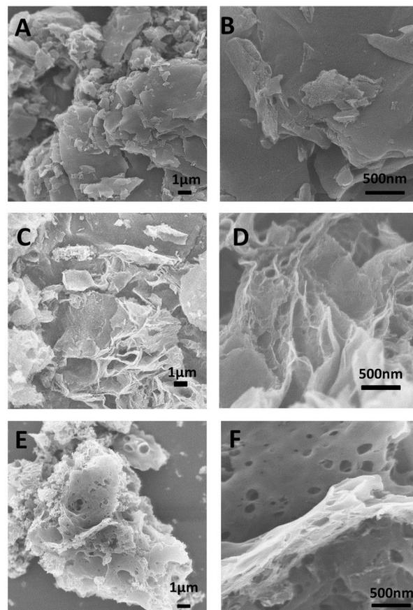
**Figure S18. SEM images of NZ<sub>0.5</sub>-C (A1, A2), NZ<sub>1</sub>-C (B1, B2) and NZ<sub>1.5</sub>-C (C1, C2).**
