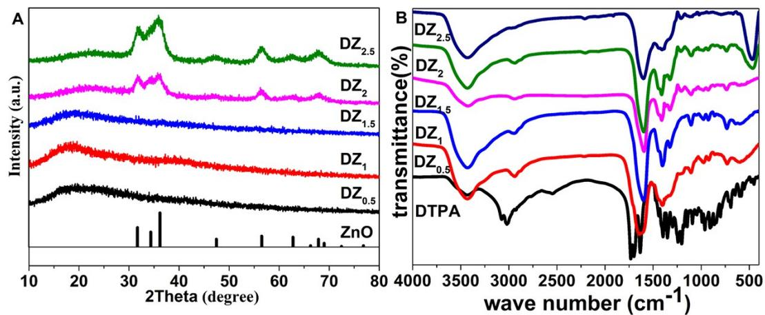
Figure S5. XRD (A) and IR (B) curves of DZ<sub>X</sub>
