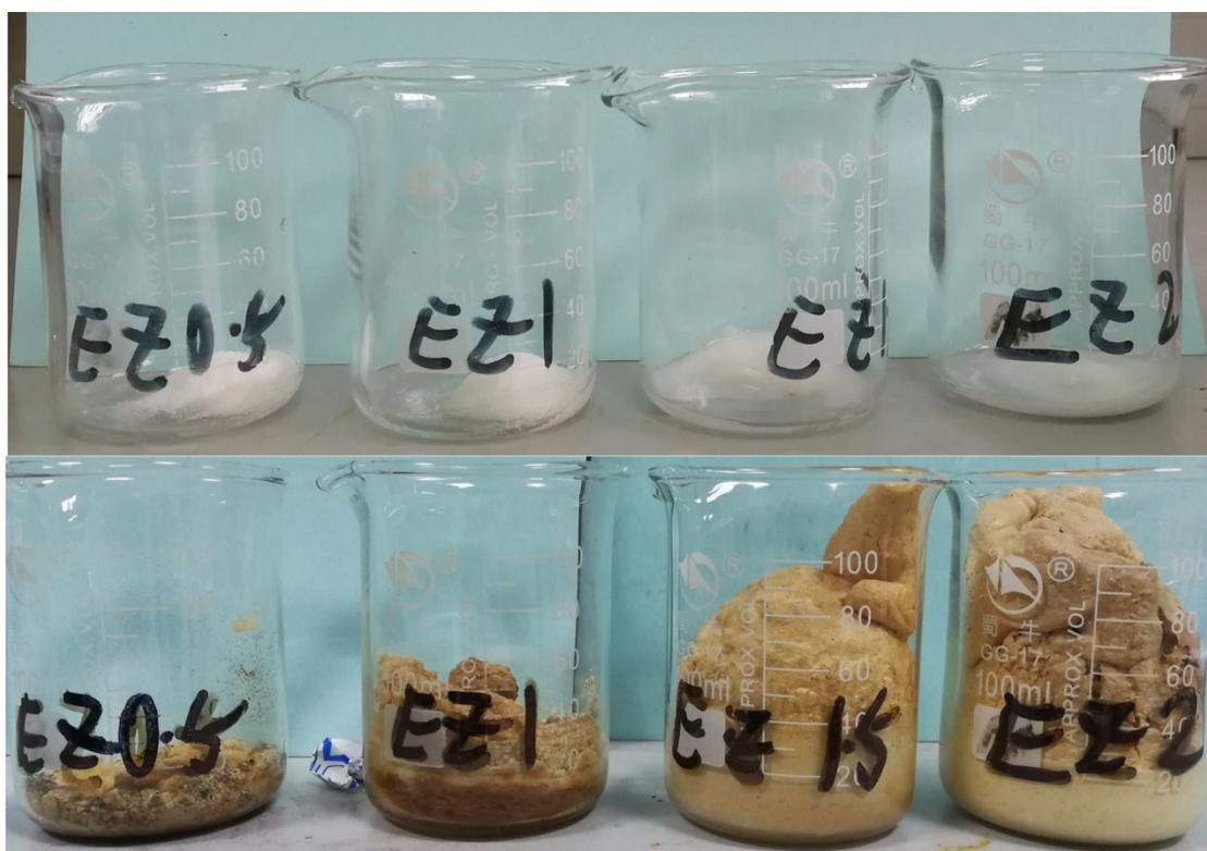
**Fig. S1. Photographs of precursors (up) and 3D Chelates Foams(down) for  $EZ_x$  in 100mL glass beaker.**
