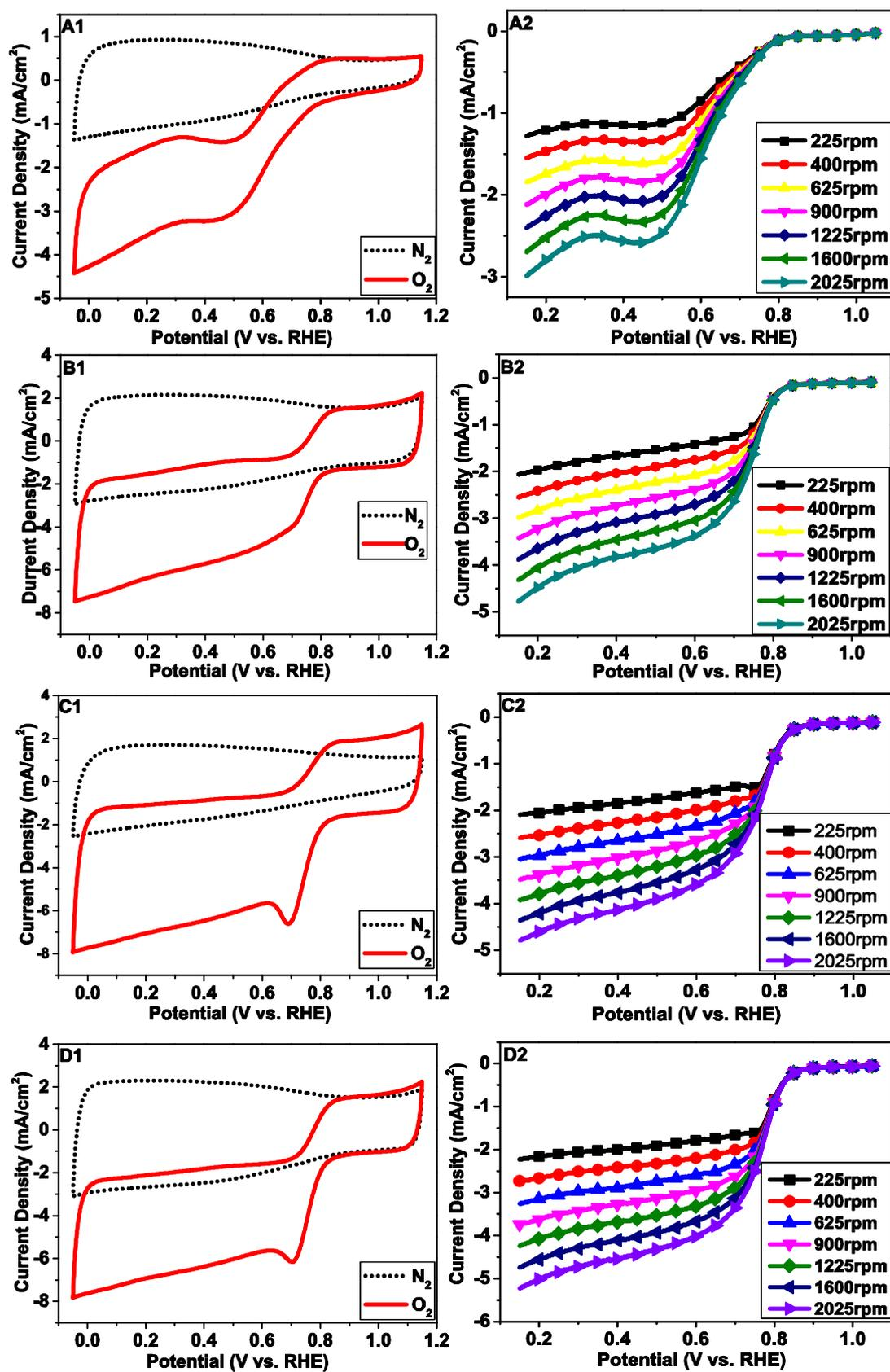
Figure S30. CV and LSV curves of  $DZ_X-C$ , A1, A2 ( $DZ_{0.5}-C$ ), B1, B2 ( $DZ_1-C$ ), C1, C2 ( $DZ_{1.5}-C$ ) and D1, D2 ( $DZ_2-C$ ).
