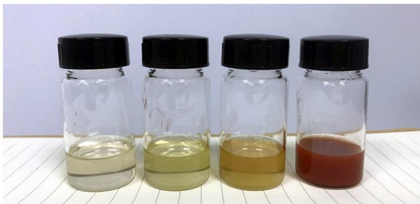
**Fig. S1** Photograph of polymer precursor solution with different SeO<sub>2</sub> addition
