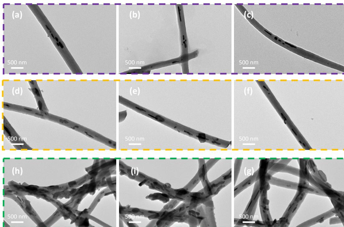
**Fig. S4** TEM images of (a-c) 10-SnSe/SnO<sub>x</sub>@CNFs, (b-f) 20-SnSe/SnO<sub>x</sub>@CNFs and (h-g) 30-SnSe/SnO<sub>x</sub>@CNFs at different positions.
