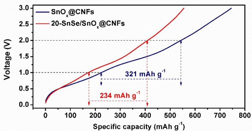
Fig. S5 The charge capacity comparison for SnO<sub>x</sub>@CNFs and 20-SnSe/SnO<sub>x</sub>@CNFs in 1.0 V - 2.0 V at 50<sup>th</sup> cycle.
