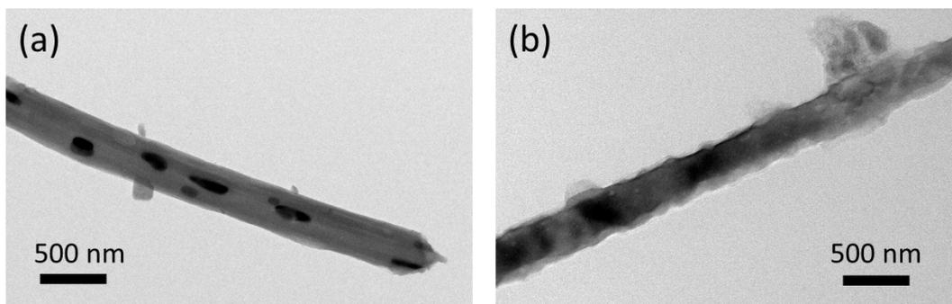
**Fig. S8** TEM image of 20-SnSe/SnO<sub>x</sub>@CNFs before (a) and after (b) 100 cycles at 1 A g<sup>-1</sup>.
