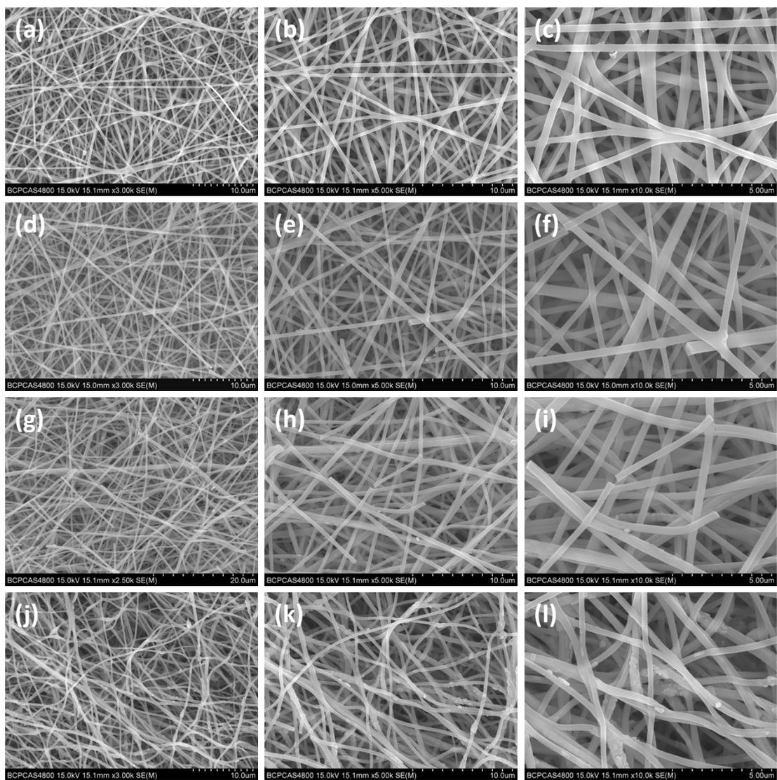
**Fig. S2** SEM images of (a-c)  $\text{SnO}_x\text{@CNFs}$ , (b-f) 10- $\text{SnSe/SnO}_x\text{@CNFs}$ , (h-i) 20- $\text{SnSe/SnO}_x\text{@CNFs}$  and (j-l) 30- $\text{SnSe/SnO}_x\text{@CNFs}$ .
