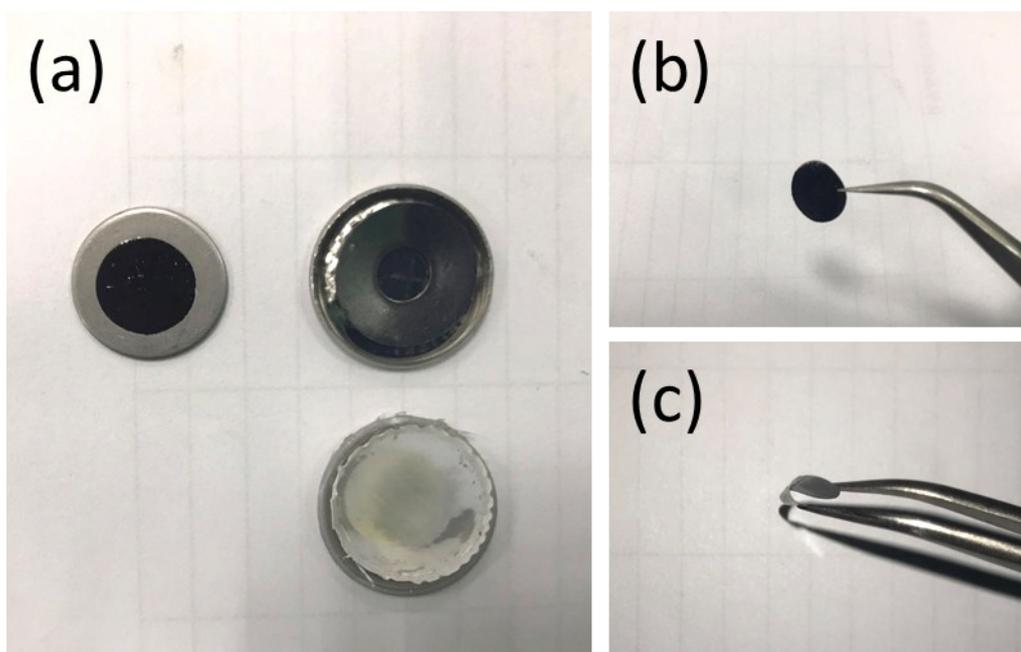
**Fig. S7** optical photograph of 20-SnSe/SnO<sub>x</sub>@CNFs electrode after 100 cycles
