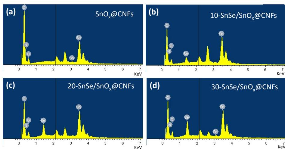
**Fig. S3** EDS spectrum of (a)SnO<sub>x</sub>@CNFs, (b)10-SnSe/SnO<sub>x</sub>@CNFs, (c)20-SnSe/SnO<sub>x</sub>@CNFs and (d)30-SnSe/SnO<sub>x</sub>@CNFs
