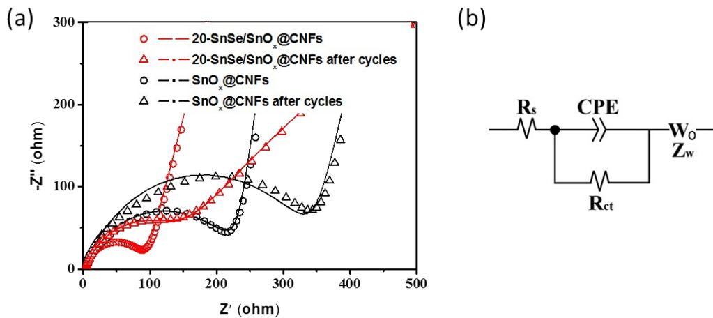
**Fig. S9** (a) EIS and fitting line for of  $\text{SnO}_x\text{@CNFs}$  and  $20\text{-SnSe/SnO}_x\text{@CNFs}$ . (b) The equivalent circuits used to fit the Nyquist plots.
