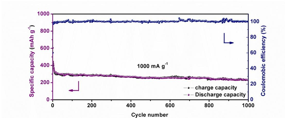
**Fig. S6** Long cycle test for SnO<sub>x</sub>@CNFs at 1000 mA g<sup>-1</sup>
