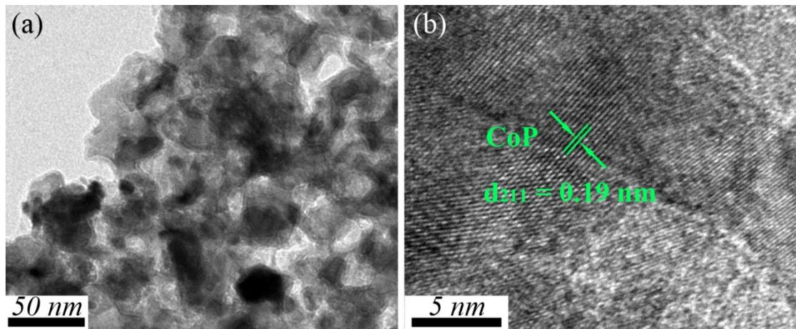
**Fig.S4** TEM (a) and HRTEM (b) images of CoP nanoparticles.
