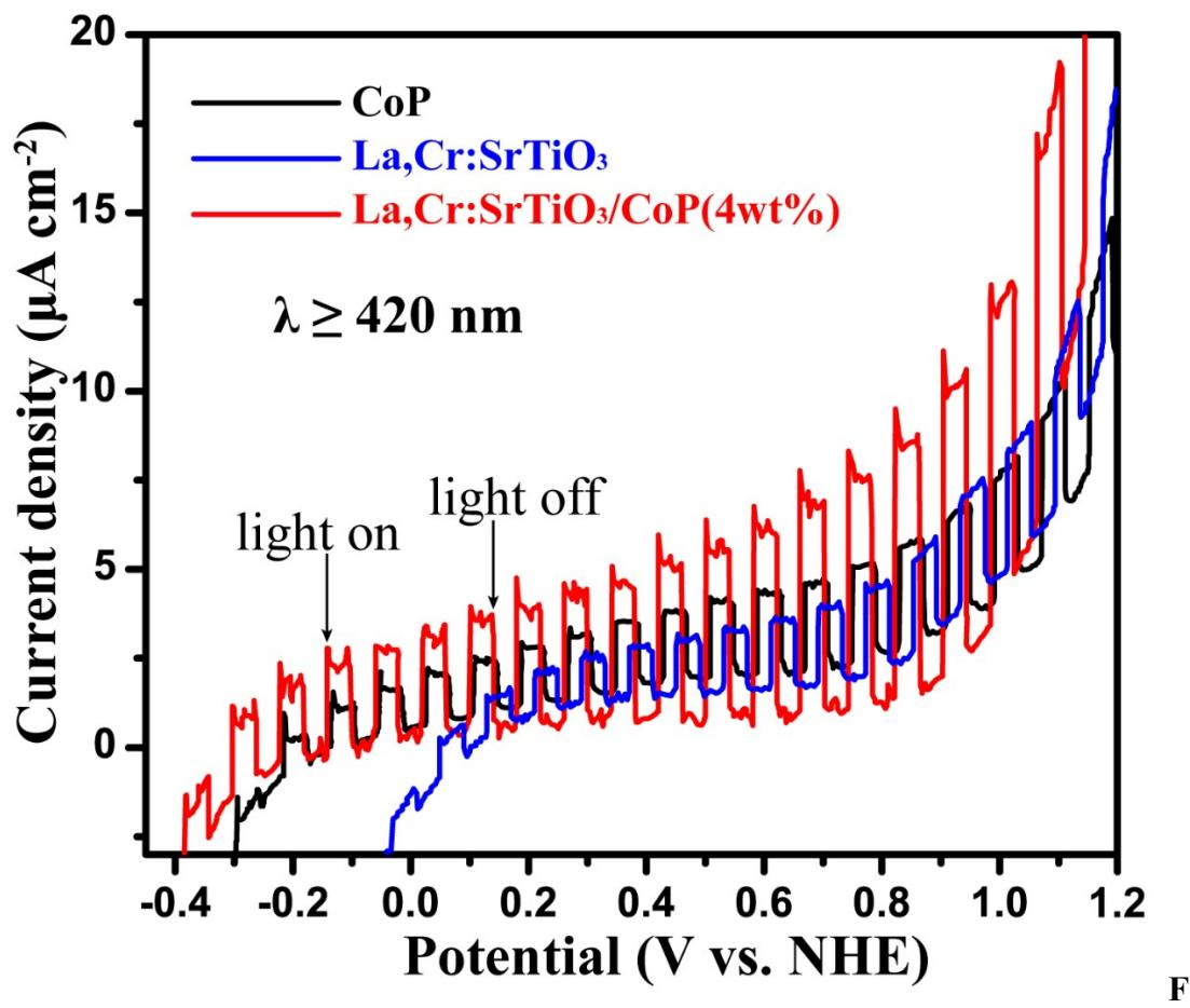
**Fig.S6** Linear sweep voltammetry (LSV) of photoelectrodes fabricated from samples CoP, La,Cr:SrTiO<sub>3</sub> and La,Cr:SrTiO<sub>3</sub>/CoP(4wt%) under chopped visible light illumination.
