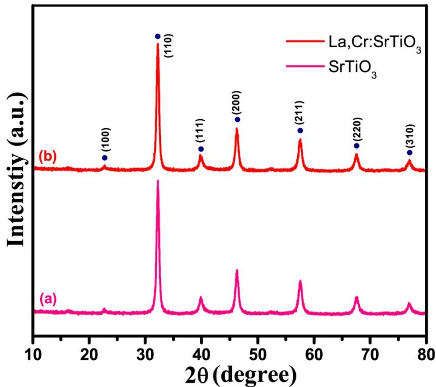
**Fig.S1** XRD patterns for SrTiO<sub>3</sub> (a) and La,Cr:SrTiO<sub>3</sub> (b).
