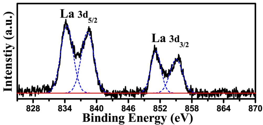
**Fig.S2** The high-resolution spectra of La 3d for La,Cr:SrTiO<sub>3</sub>/CoP(4wt%) sample.
