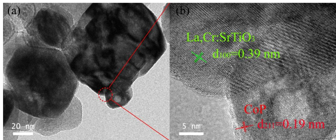
**Fig.S5** TEM (a) and HRTEM (b) images of  $\text{La,Cr:SrTiO}_3/\text{CoP}(4\text{wt}\%)$  composite.
