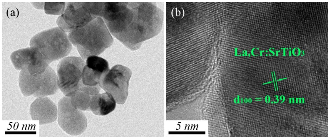
**Fig.S3** TEM (a) and HRTEM (b) images of  $\text{La,Cr:SrTiO}_3$  nanoparticles.
