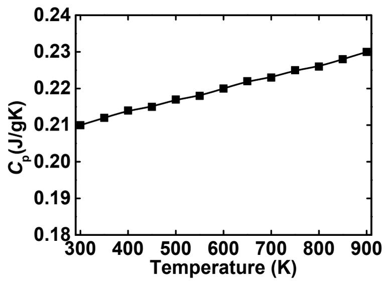
**Figure S1** The used heat capacity,  $C_p$ , of each sample, which was estimated by the relationship  $C_p (K_B \text{ Per atom}) = 3.07 + 4.7 \times 10^{-4} \times (T/K - 300)$ .
