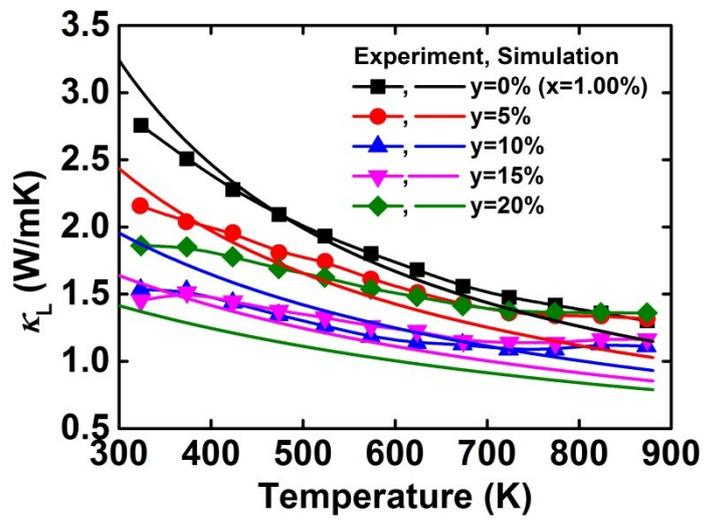
**Figure S4** Lattice thermal conductivities of  $\text{Sn}_{0.99}\text{In}_{0.01}\text{Te}_{1-y}\text{Se}_y$  (Figure 8(b)) and theoretical thermal conductivities by the Debye-Callaway model.
