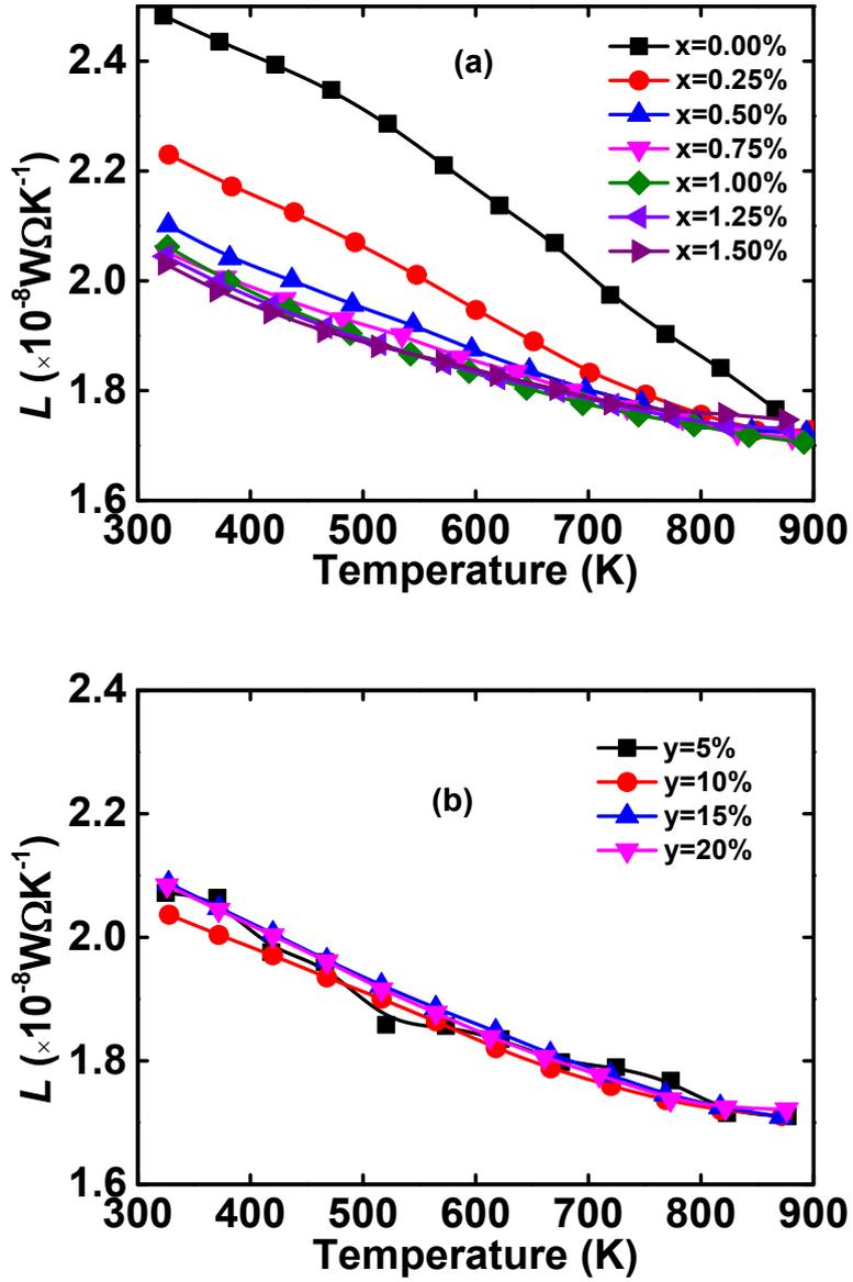
**Figure S3** The Lorenz number,  $L$ , for  $\text{Sn}_{1-x}\text{In}_x\text{Te}$  (a), and  $\text{Sn}_{0.99}\text{In}_{0.01}\text{Te}_{1-y}\text{Se}_y$  alloys (b), which were derived from the equation of  $L=1.5+\exp(-|S|/116)$ .
