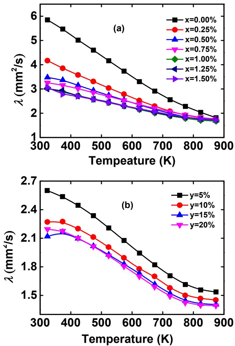
**Figure S2** Thermal diffusivity,  $\lambda$ , for  $\text{Sn}_{1-x}\text{In}_x\text{Te}$  (a), and  $\text{Sn}_{0.99}\text{In}_{0.01}\text{Te}_{1-y}\text{Se}_y$  alloys (b).
