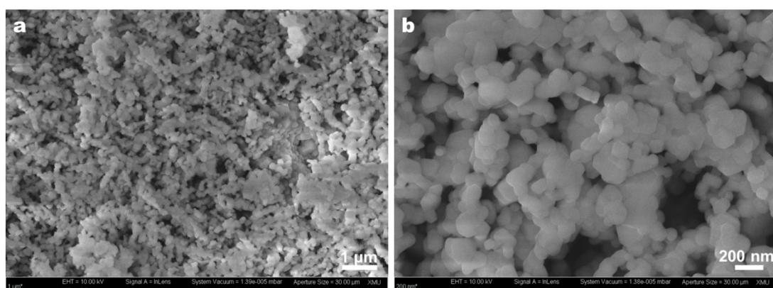
**Figure S2.** (a) Low-magnification SEM image, and (b) high-magnification SEM image of the nanoparticles obtained by directly sintering the PAN/metal acetates nanofibres to 750 °C.
