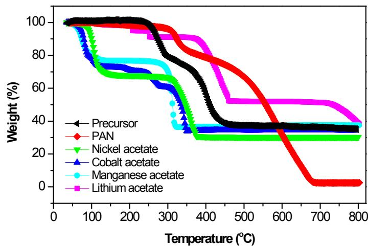
**Figure S4.** TGA curves of the electrospun PAN/NCM composite precursor, PAN and metal acetates.
