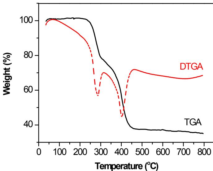
**Figure S3.** TGA-DTGA curves of the electrospun PAN/NCM composite nanofibres.
