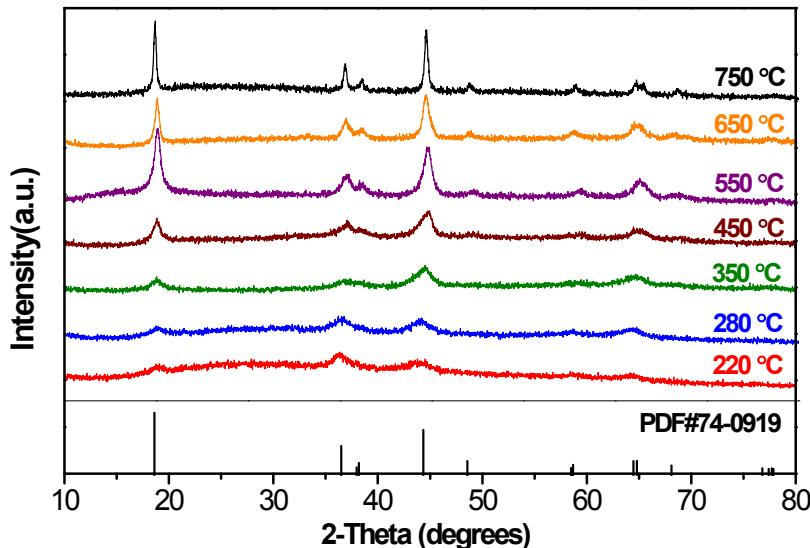
**Figure S4.** XRD patterns of the samples obtained at different temperatures.
