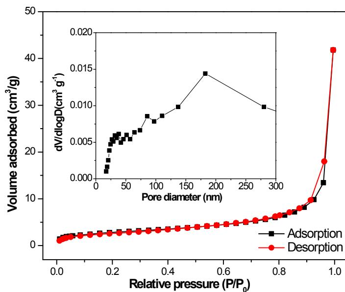
**Figure S7.** Nitrogen adsorption/desorption isotherms and the corresponding pore size distribution for the Nb-NCM nanobelts.
