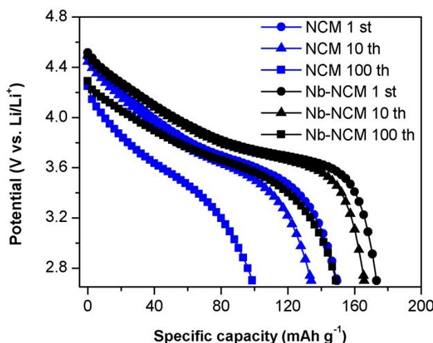
**Figure S6.** Discharge curves of Nb-NCM and NCM electrodes at 1 C.
