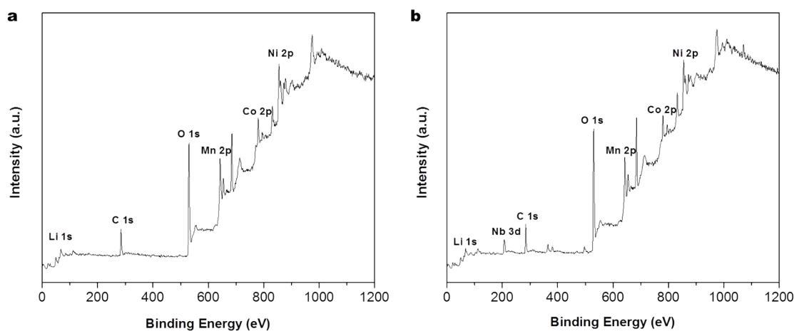
**Figure S5.** The wide XPS spectra of (a) NCM nanobelts, and (b) Nb-NCM nanobelts.
