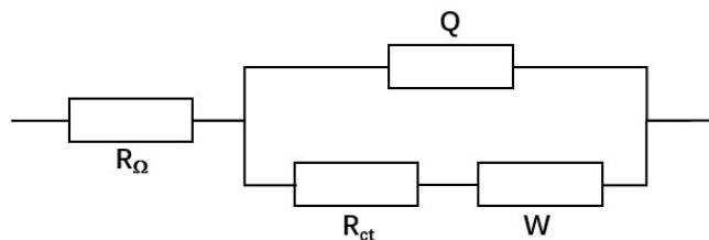
**Figure S8.** The simplified equivalent circuit of the Nb-NCM nanobelts and NCM nanobelts.
