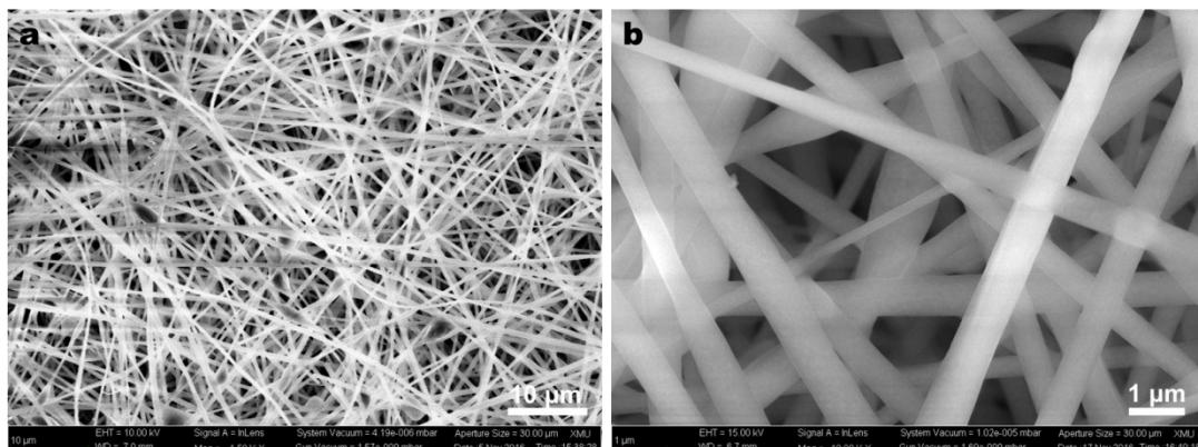
**Figure S1.** (a) Low-magnification SEM image, and (b) high-magnification SEM image of the as-electrospun PAN/metal acetates nanofibres.
