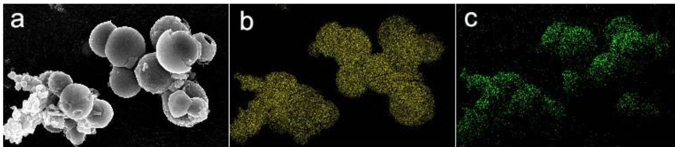
**Fig. S1.** SEM image of the VO<sub>2</sub>(D)-HCSMs (a) and their mapping images of V (b) and O (c).
