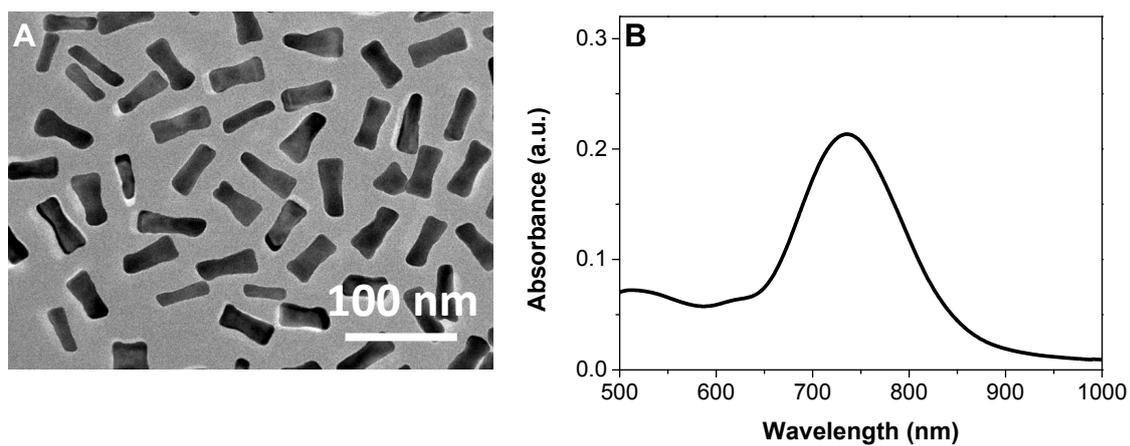
**Figure S3.** (A) TEM image of Au nanorods. (B) UV-vis absorption spectrum of Au nanorods.
