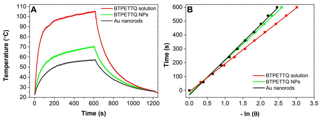
**Figure S5.** (A) Temperature changes of BTEPTTQ solution, NPs and Au nanorods with a concentration of 100  $\mu\text{g}/\text{mL}$ , in which the laser is switched off after 10 min irradiation. (B) Plot of time starting from the cooling stage versus negative natural logarithm of drive force temperature. The slop represents the sample system time constant  $\tau_s$ .
