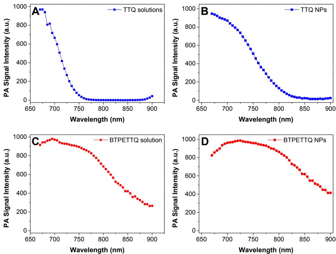
**Figure S2.** PA signal intensity of TTQ solution (A), NPs (B), BTPETTQ solution (C) and NPs (D) upon laser excitation at different wavelengths from 670 nm to 900 nm.
