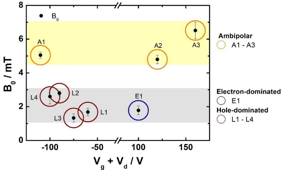
E1:  $V_g = 70$  V,  $V_d = 30$  V    L1:  $V_g = -40$  V,  $V_d = -20$  V    L2:  $V_g = -70$  V,  $V_d = -20$  V
