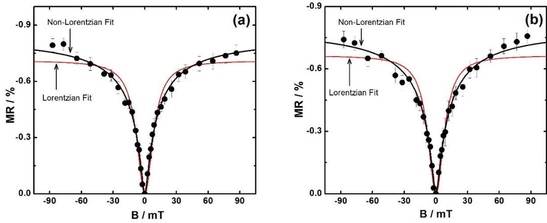
**Fig. S3** Representative MR(B) line shape curves based on magnetotransport measurements performed for two different voltage conditions: (a) Point A1:  $V_d = -90$  V and  $V_g = -20$  V and (b) Point A3:  $V_d = 70$  V and  $V_g = 90$  V. These points can also be found in the main text, as displayed in Figures 3 and 6. The black lines show the Non-Lorentzian fittings and the red lines show the Lorentzian fittings.
