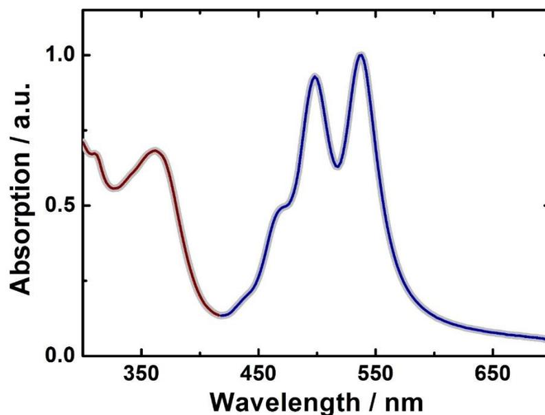
**Fig. S1** Absorption spectrum of a 35 nm-thin evaporated film of Spiro-DPASP-*t*Bu-Phenyl on a glass substrate. The spectrum is composed of the spectrally separated absorption bands of the donor-like spiro-substituted diphenylamine (red) and the acceptor-like perylenetetracarboxylicdiimide-derivative chromophore (blue).
