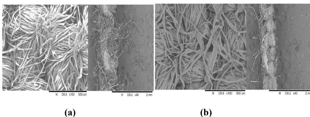
**Figure S1** Surface morphology (left) and cross section (right) of (a) uncoated (b) SMPU coated fabric.
