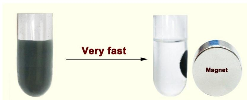
**Figure S1.** The illustration for the magnetic separation of catalysts after reaction.
