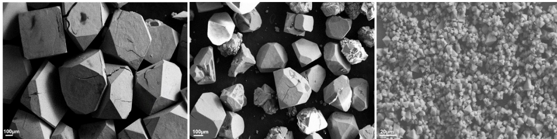
Figure S8. SEM images of Cu/Zn@C materials with different particle sizes. From left to right: Cu/Zn@C-mm, Cu/Zn@C-submm, and Cu/Zn@C-μm.
