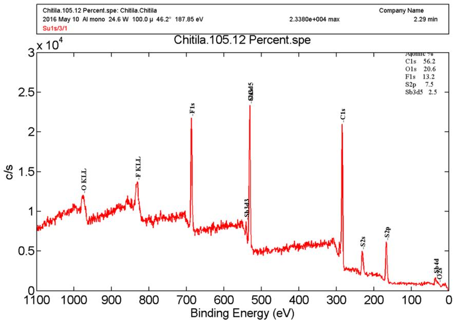
**Figure S15.** Area scans X-ray photoelectron spectra (XPS) profile of 2.15% MAPDSA-MAPDST copolymer.
