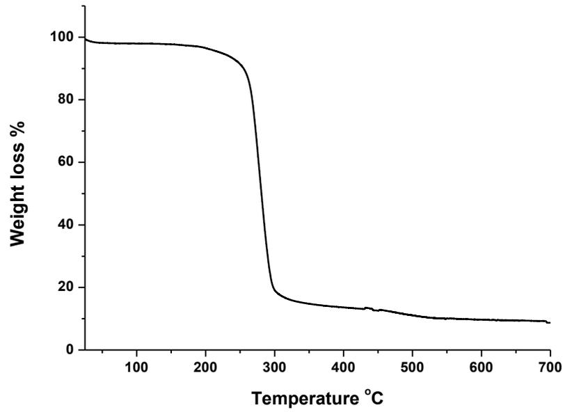
**Figure S12.** TGA profile of 1.5% MAPDSA-MAPDST copolymer.
