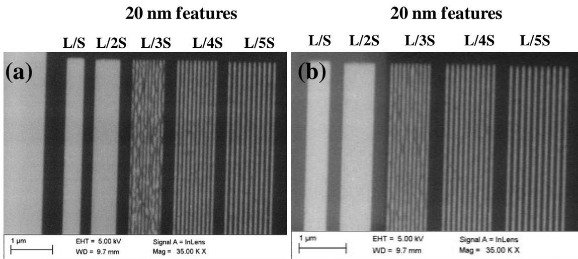
**Figure S18.** FE-SEM images of EUV exposed MAPDSA-MAPDST hybrid resist patterns: (a) 20 nm line features with L/S to L/5S (line/space) characteristics of 1.5 % resist; (b) 20 nm line features with L/S to L/5S (line/space) characteristics of 2.15 % resist.
