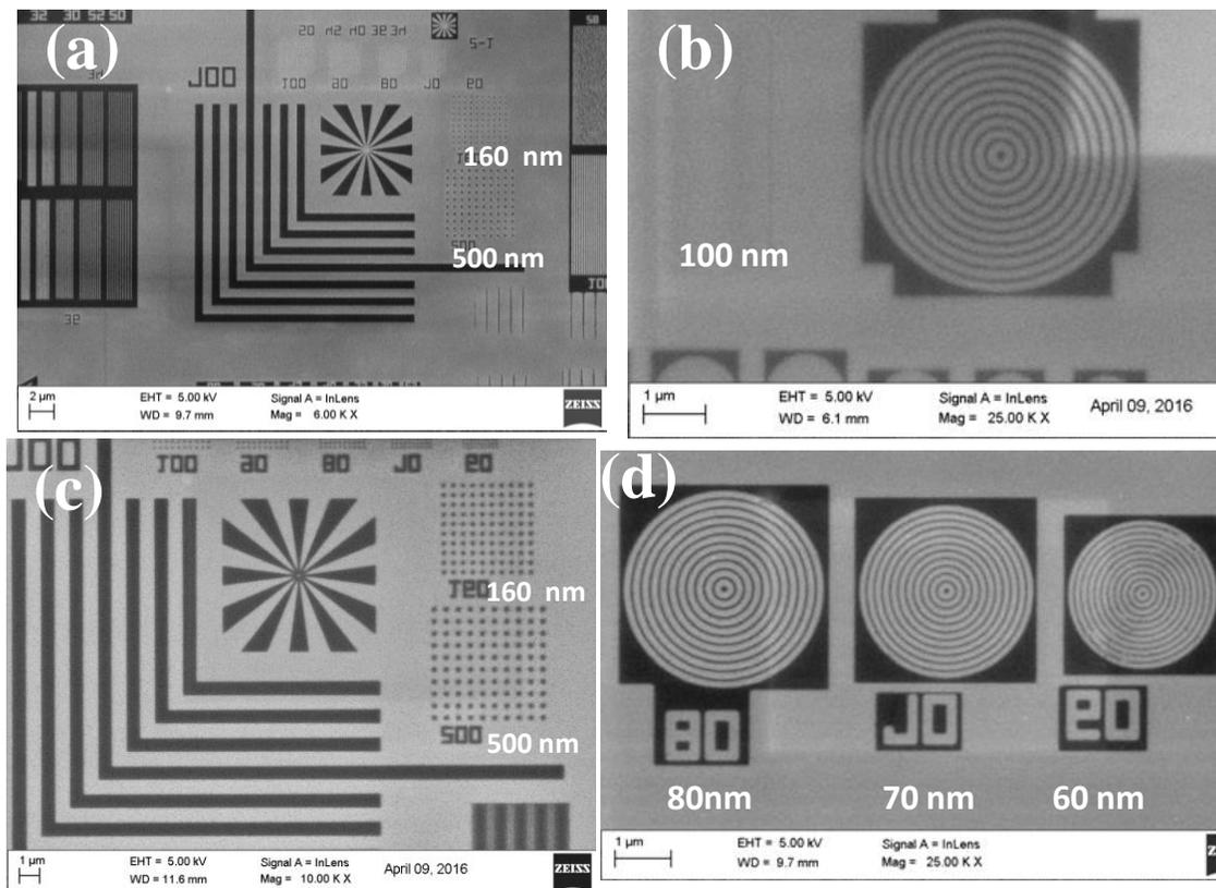
**Figure S20.** FE-SEM images of EUV exposed MAPDSA-MAPDST hybrid resist patterns: (a) Star elbow features with nano-dots (500 and 160 nm) of 1.5 % resist; (b) 100 nm ring patterns of 1.5 % resist; (c) Star elbow features with nano-dots (500 and 160 nm) of 2.15 % resist; (d) 80, 70 and 60 nm rings of 2.15 % resist.
