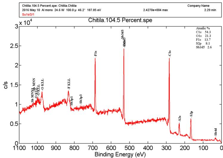
**Figure S14.** Area scans X-ray photoelectron spectra (XPS) profile of 1.5% MAPDSA-MAPDST copolymer.
