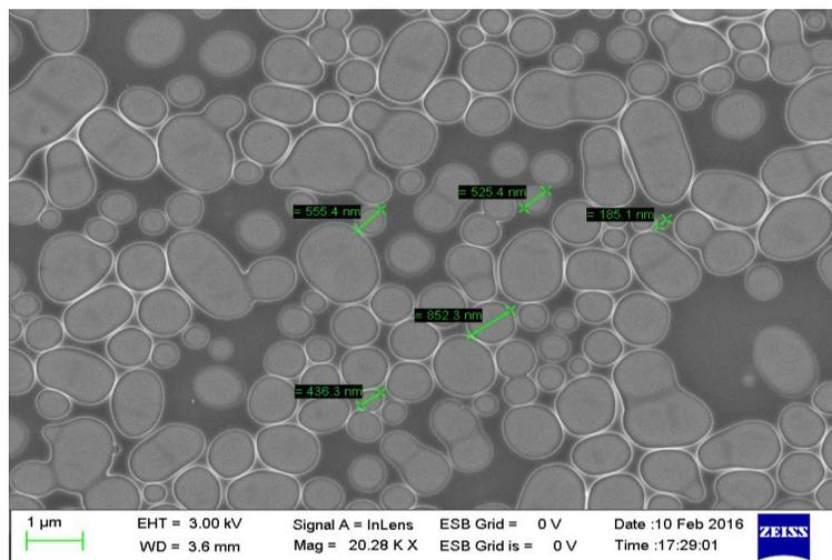
**Figure S16.** FE-SEM image of thin film obtained by spin coating of MAPDSA-MAPDST (50:50 feed ratio) copolymer resist in acetonitrile solvent.
