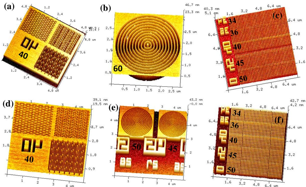
**Figure S19.** AFM-3D image of EUV exposed complex nano-features: (a) 40 nm boats, waves and line-elbow connections of 1.5 % resist; (b) 60 nm circular patterns of 1.5 % resist; (c) 50-34 nm dots of 1.5 % resist; (d) 40 nm boats, waves and line-elbow connections of 2.15 % resist; (e) 45 and 50 nm circular patterns of 2.15 % resist; (f) 50-34 nm dots of 2.15 % resist.
