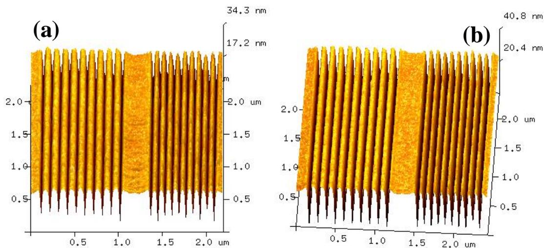
**Figure S17.** AFM 3-D view of EUV exposed MAPDSA-MAPDST hybrid resist patterns: (a) Higher resolution 20 nm (L/4S and L/3S) line features of 1.5 % resist; (b) higher resolution 20 nm (L/4S and L/3S) line features of 2.15 % resist.
