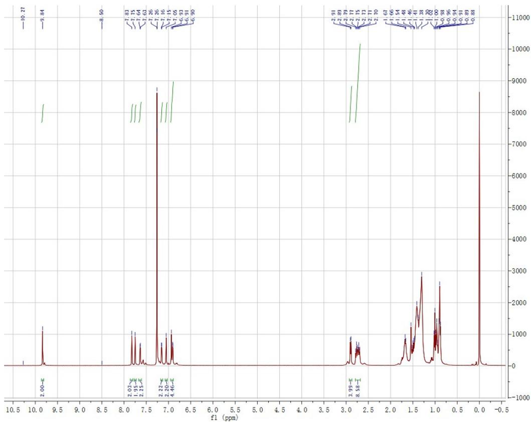
**Figure S2.**  $^1\text{H-NMR}$  spectrum of **NDTCHO** in  $\text{CDCl}_3$ .
