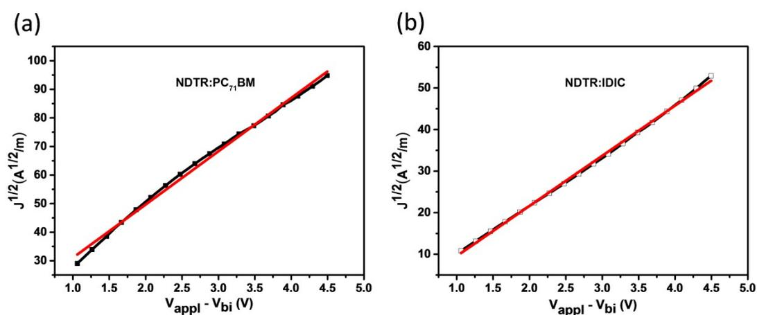
**Figure S5.** The corresponding  $J^{1/2}$ - $V$  curves for hole-only devices composed of donor/acceptor in the dark.
