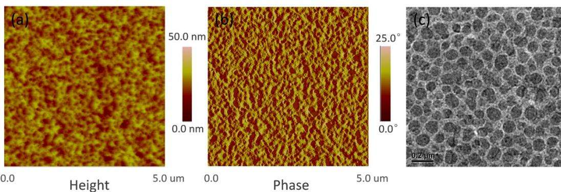
**Figure S7.** The AFM and TEM images of NDTR:PC<sub>71</sub>BM system without DPE as additive.
