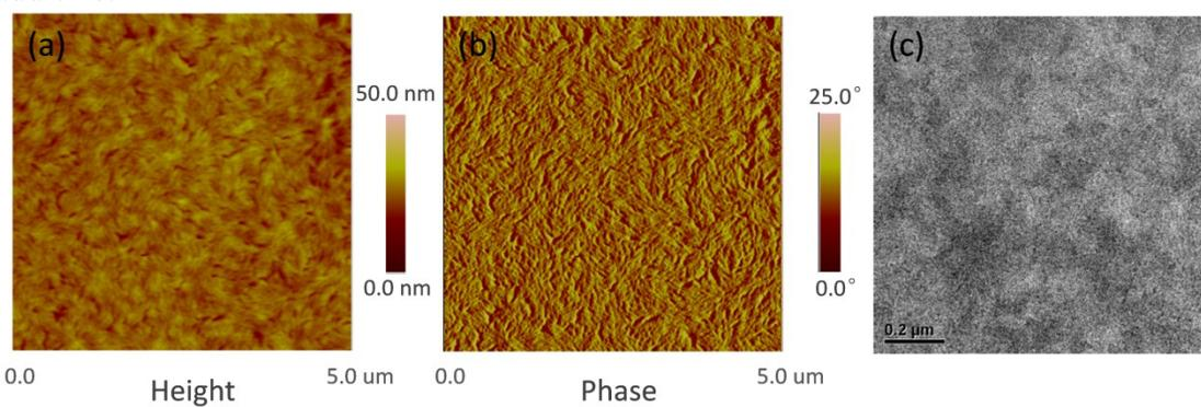
**Figure S8.** The AFM and TEM images of NDTR:IDIC system without thermal annealing (TA).
