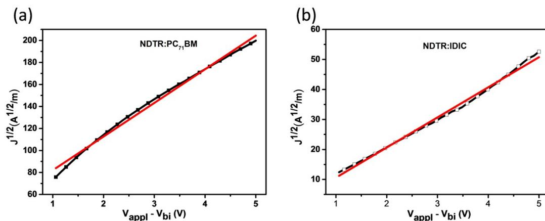
**Figure S6.** The corresponding  $J^{1/2}$ - $V$  curves for electron-only devices composed of donor/acceptor in the dark.
