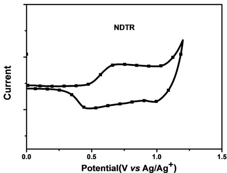
**Figure S4.** Electrochemical cyclic voltammetry curve of the NDTR film measured in  $0.1 \text{ mol L}^{-1} \text{ Bu}_4\text{NPF}_6$  acetonitrile solutions
