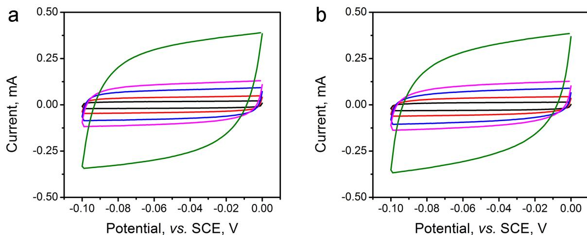
**Fig. S13.** ECSA measurements of (a) ZiF-8-C4 and (b) ZiF-8-C6 after the 8-hour electrolysis test in 0.1 M KOH.
