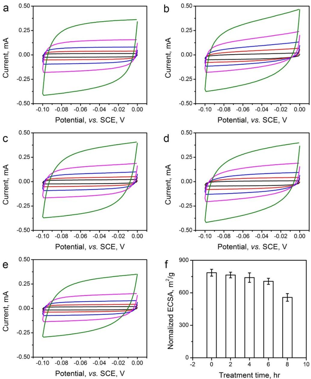
**Fig. S11.** Cyclic voltammetry (CV) scan curves of ZIF-8-C0~C8. The scan rates vary from 5 to 50 mV/s. (f) The calculated ECSA values for ZIF-8-C0~C8.
