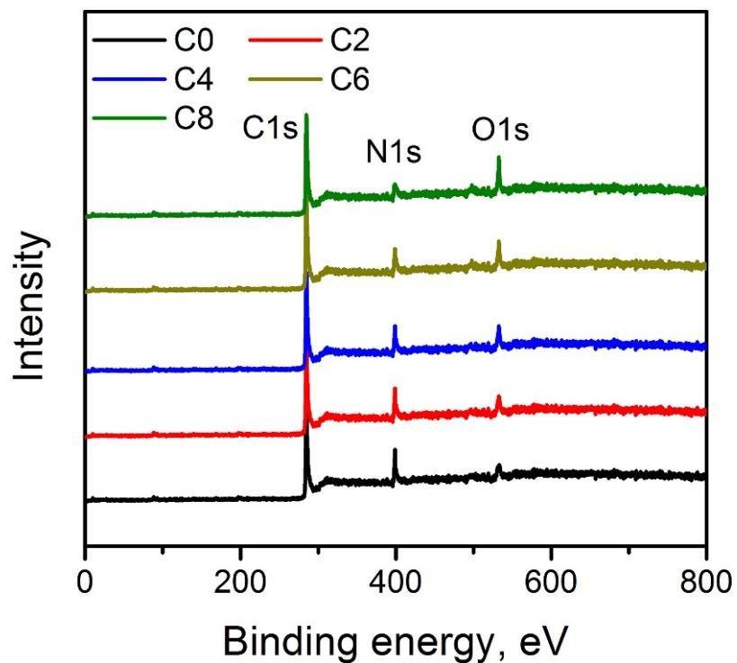
**Fig. S3.** XPS survey scans of ZIF-8 derived carbon materials upon the cathodic polarization treatment in 0.5 M H<sub>2</sub>SO<sub>4</sub> over the different periods of time.
