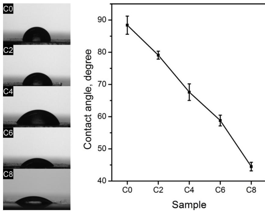
**Fig. S2.** Contact angle measurement of ZIF-8-C0~C8. (Left) photos and (right) contact angles.
