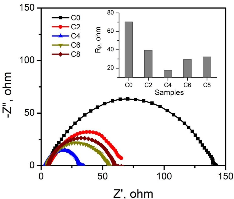
**Fig. S8.** EIS Nyquist plots of the ZIF-8-derived electrocarbocatalysts for OER in 0.1 M KOH electrolyte. All plots are recorded with the overpotential of 0.3 V. The insert shows the polarization resistance ( $R_p$ ).
