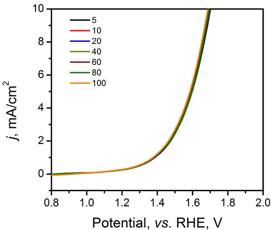
**Fig. S9.** OER LSV curve of ZIF-8-C4 obtained at the different scan rates (from 5 to 100 mV/s) in 0.1 M KOH electrolyte.
