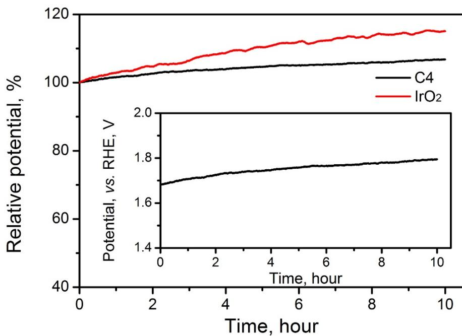
**Fig. S10.** The relative potentials of ZIF-8-C4 and IrO<sub>2</sub> catalysts in the OER tests carried out at 10 mA/cm<sup>2</sup> in 0.1 M KOH electrolyte for 10 hours. The inset shows the chronoamperometric curve of ZIF-8-C4.
