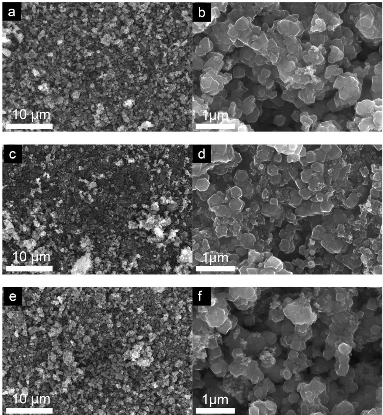
**Fig. S1.** SEM images of (a–b) ZnF-8-C2, (c–d) ZnF-8-C4, and (e–f) ZnF-8-C8 carbon materials at the different magnifications.
