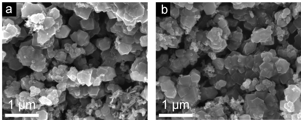
**Fig. S12.** SEM images of (a) ZiF-8-C4 and (b) ZiF-8-C6 after the 8-hour electrolysis test in 0.1 M KOH.
