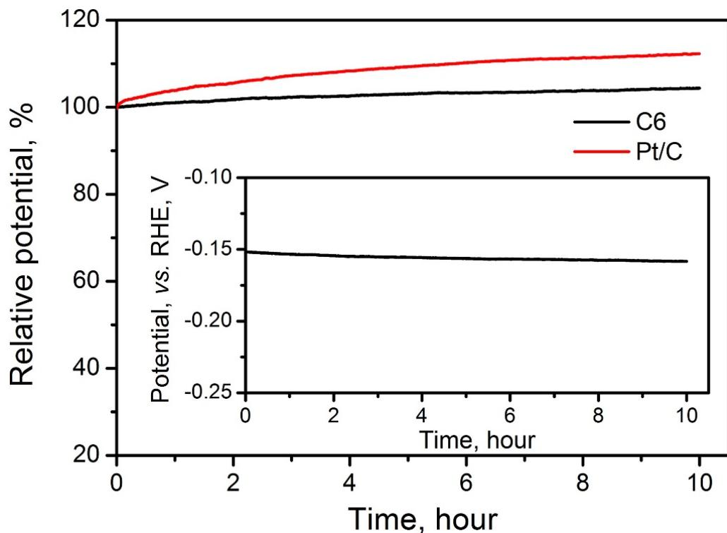
**Fig. S7.** The relative potentials of ZIF-8-C6 and Pt/C electrocatalysts in the HER tests carried out at 10 mA/cm<sup>2</sup> in 0.5 M H<sub>2</sub>SO<sub>4</sub> electrolyte for 10 hours. The inset shows the chronoamperometric curve of ZIF-8-C6.
