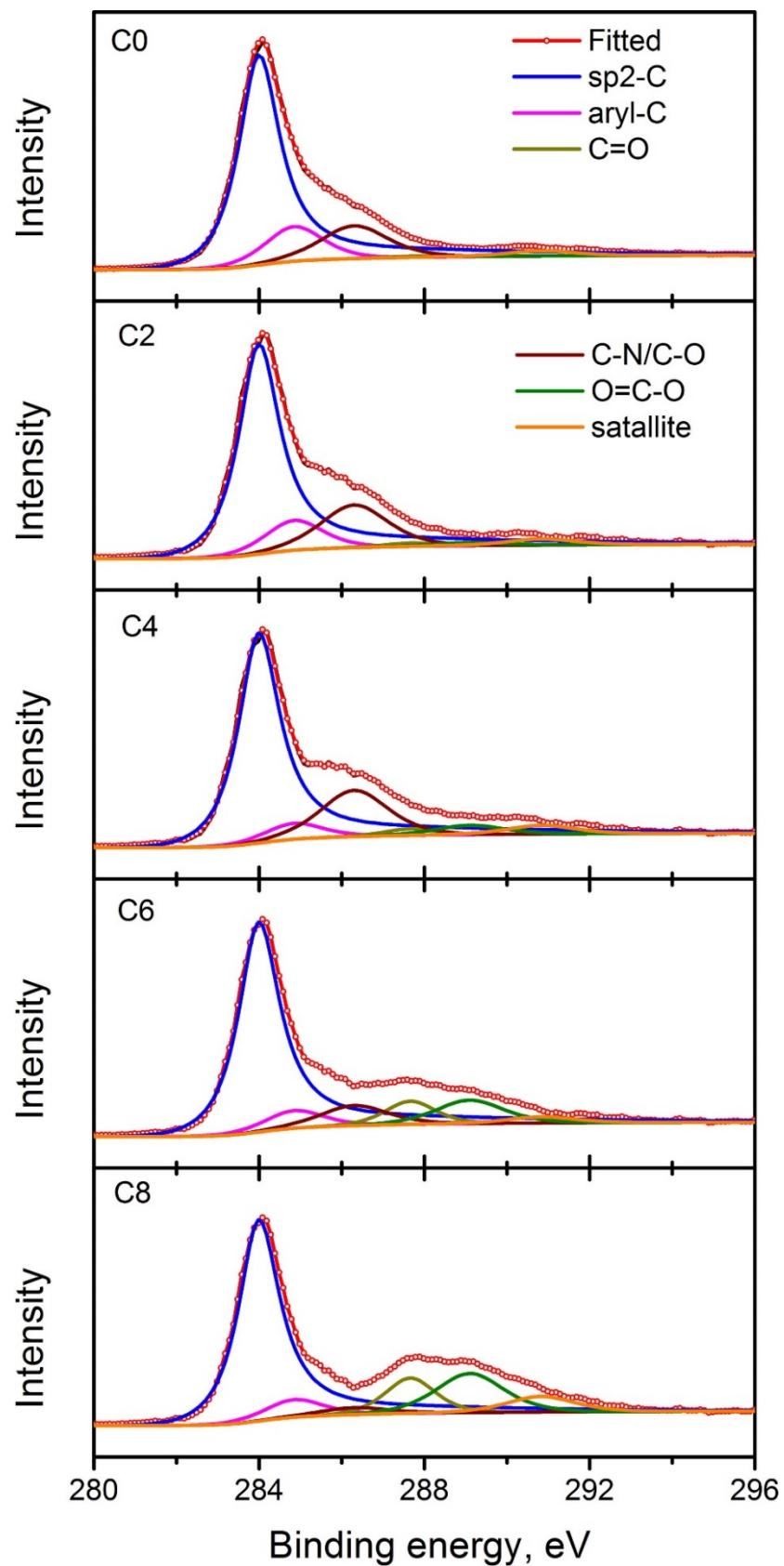
**Fig. S4.** Deconvolution of the high-resolution XPS spectra of C in the ZIF-8 derived carbon materials.
