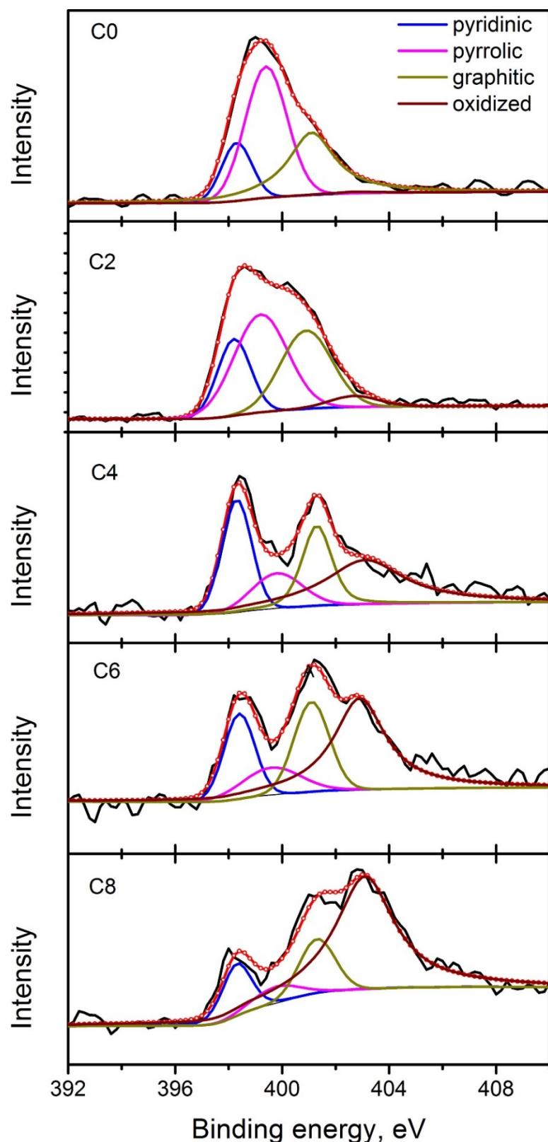
**Fig. S5.** Deconvolution of the high-resolution XPS spectra of N in the ZIF-8-derived carbon materials.
