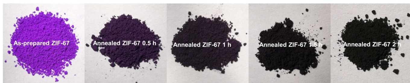
Figure S4. The color changes of the ZIF-67 samples after annealing in N_2 at 450\text{ }^\circ\text{C} for different durations.
