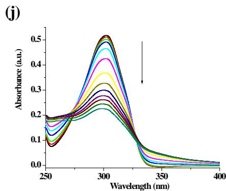
**Fig. S35.** Change in absorbance of **2** ( $c = 2.5 \times 10^{-5}$  M) upon addition of 10 equiv. amount of (a)  $\text{Pb}^{2+}$ , (b)  $\text{Mg}^{2+}$ , (c)  $\text{Co}^{2+}$ , (d)  $\text{Ni}^{2+}$ , (e)  $\text{Zn}^{2+}$ , (f)  $\text{Cd}^{2+}$ , (g)  $\text{Fe}^{2+}$ , (h)  $\text{Hg}^{2+}$ , (i)  $\text{Cu}^{2+}$ , (j)  $\text{Ag}^+$  ( $c = 1.0 \times 10^{-3}$  M) in DMSO:  $\text{H}_2\text{O}$  (1:9, v/v).
