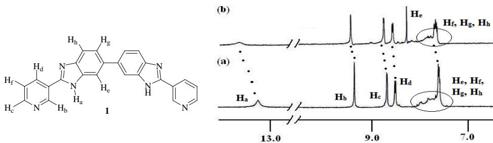
**Fig. S38.** <sup>1</sup>H NMR (400 MHz, *d*<sub>6</sub>-DMSO) of (a) compound **1** (*c* = 1.50 × 10<sup>-2</sup> M) and (b) **1** with equiv. amount of AgClO<sub>4</sub>.
