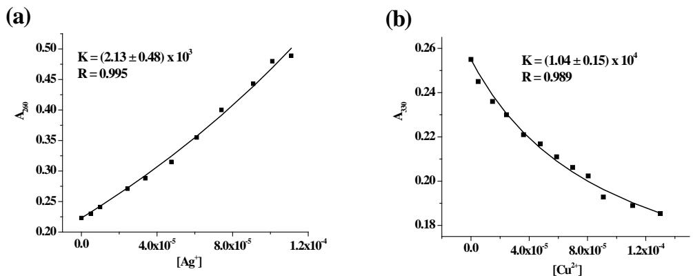
**Fig. S34.** Non liner binding constant curve for **1** ( $c = 2.5 \times 10^{-5}$  M) with (a)  $\text{Ag}^+$  and (b)  $\text{Cu}^{2+}$  ( $c = 1.0 \times 10^{-3}$  M) in DMSO:  $\text{H}_2\text{O}$  (1:9, v/v) from UV.
