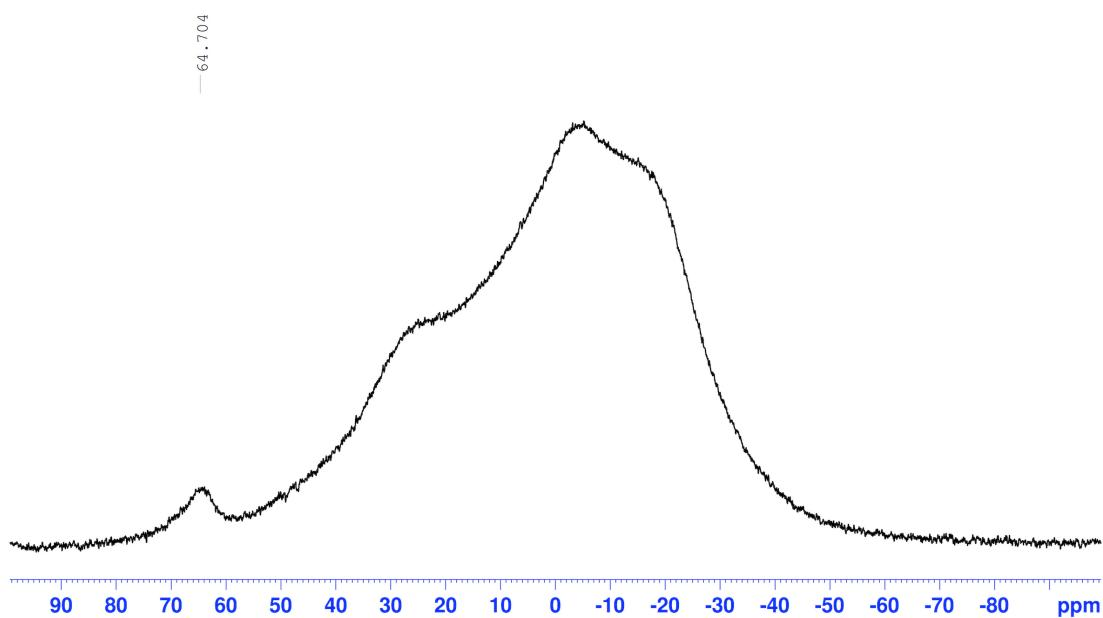
**Fig. S7.** <sup>11</sup>B NMR spectrum (128 MHz) of **1tBu** in  $\text{CDCl}_3$  at 25 °C. The broad peaks in a region from 50 to -40 ppm are the contributions from a borosilicate-glass NMR tube.
