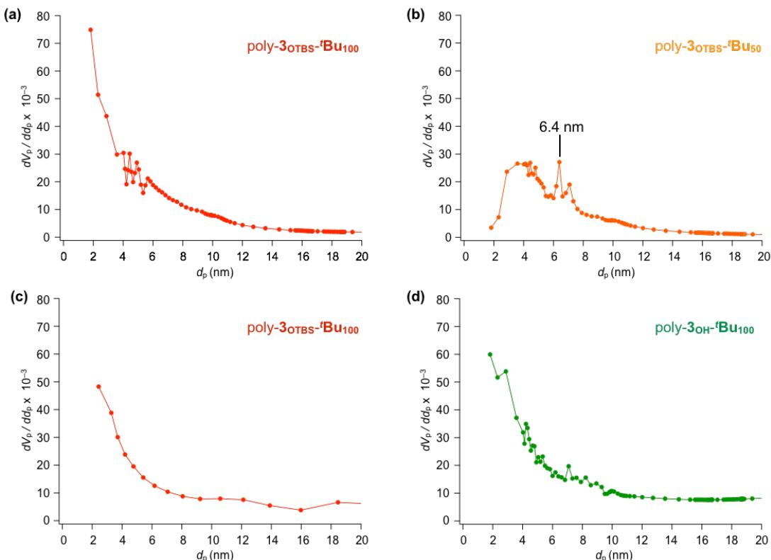
**Fig. S4.** BJH pore size distribution profiles of powder samples of (a) poly- $\mathbf{3OTBS-\text{'Bu}_{100}}$  and (b) poly- $\mathbf{3OTBS-\text{'Bu}_{50}}$  obtained from poly- $\mathbf{2OTBS}$  ( $M_n = 6,400$ , PDI = 2.02), and (c) poly- $\mathbf{3OTBS-\text{'Bu}_{100}}$  and (d) poly- $\mathbf{3OH-\text{'Bu}_{100}}$  obtained from poly- $\mathbf{2OTBS}$  ( $M_n = 5,900$ , PDI = 2.02).
