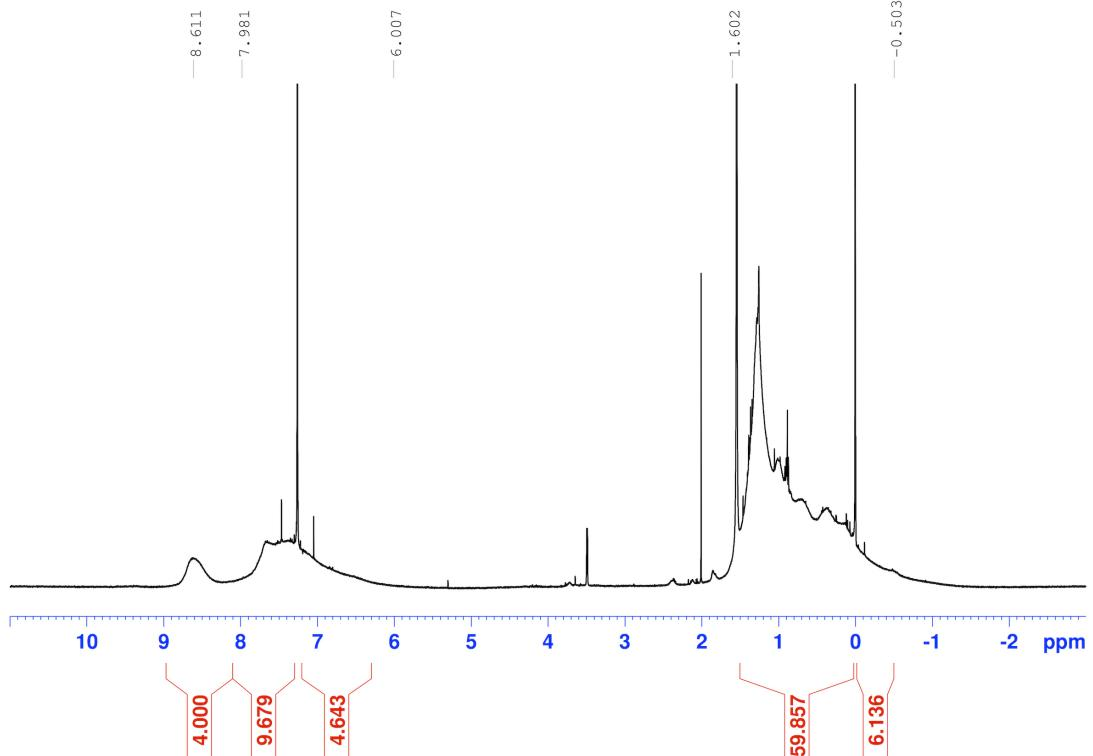
**Fig. S13.**  $^1\text{H}$  NMR spectrum (500 MHz) of poly-3OTBS- $'\text{Bu}_{100}$  in  $\text{CDCl}_3$  at 25 °C.
