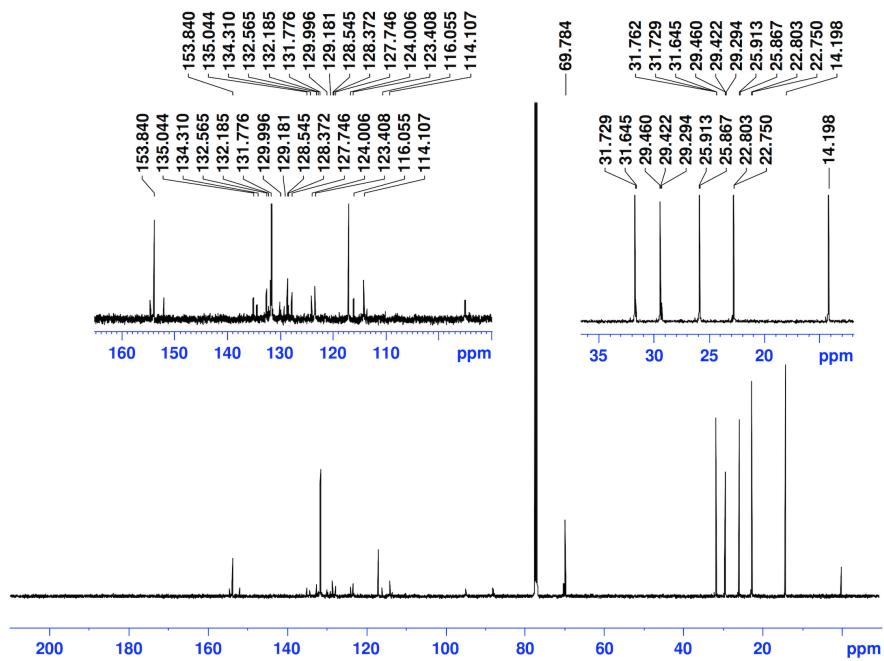
**Fig. S12.**  $^{13}\text{C}$  NMR spectrum (125 MHz) of poly-**1**<sub>OHex</sub> in  $\text{CDCl}_3$  at 25 °C.
