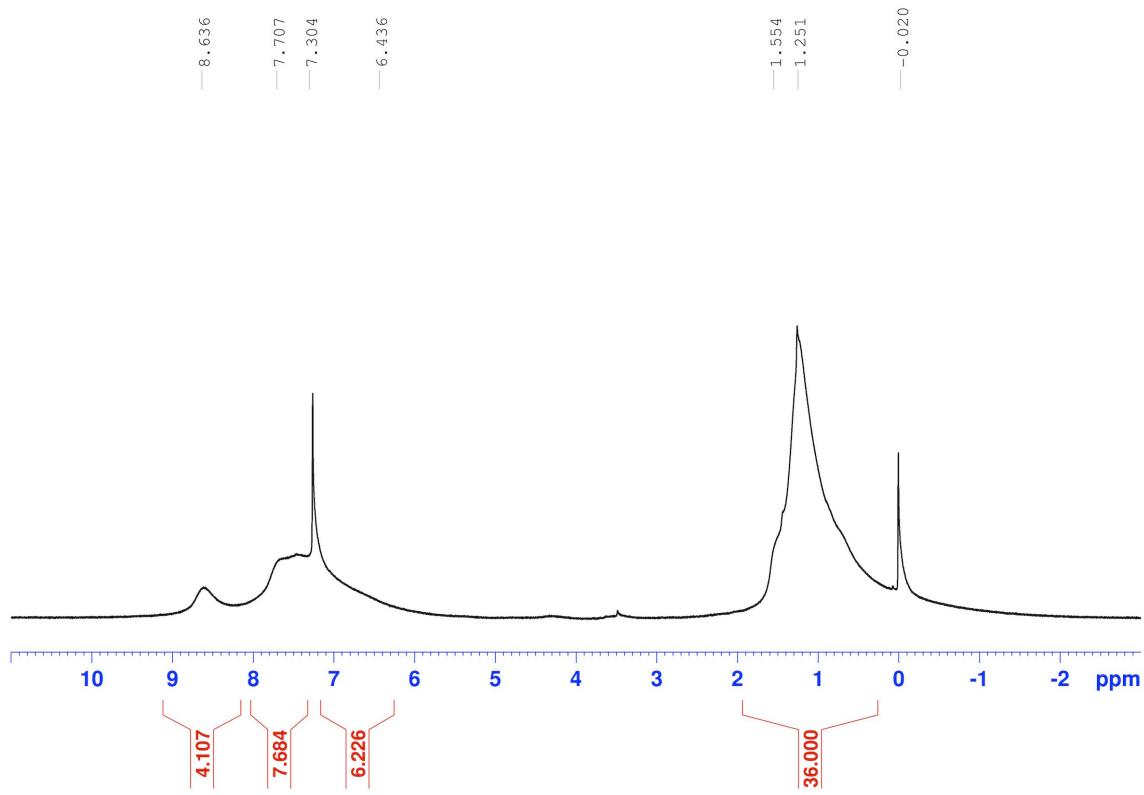
**Fig. S22.** <sup>1</sup>H NMR spectrum (500 MHz) of poly-3OH-<sup>t</sup>Bu<sub>100</sub> in CDCl<sub>3</sub> at 25 °C.
