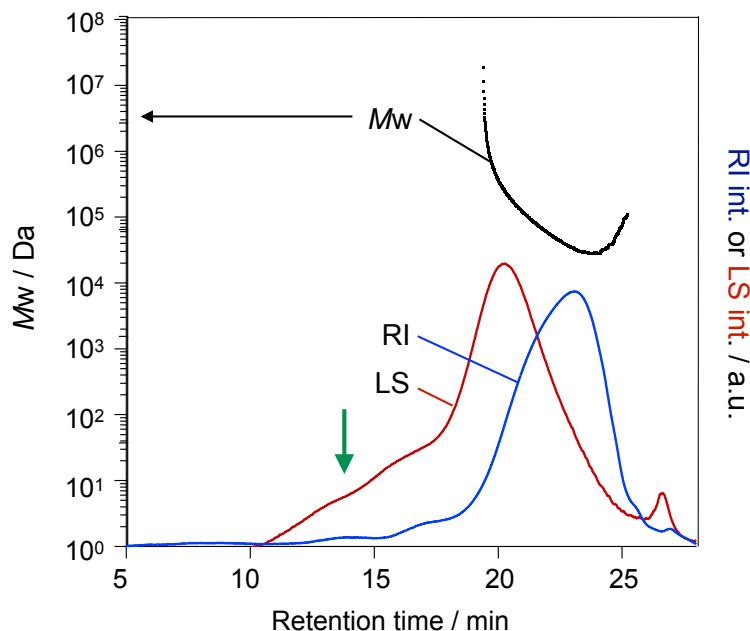
**Fig. S3.** SEC-MALS profile of poly- $\mathbf{3OTBS-\text{'Bu}_{100}}$  ( $M_n = 4.77 \times 10^4$  Da, PDI = 1.66). The observed rise in the light-scattering (LS) trace (green arrow) suggests the occurrence of polymer aggregation in the SEC analysis, which may lead to the overestimation of the molecular weight of the polymer.
