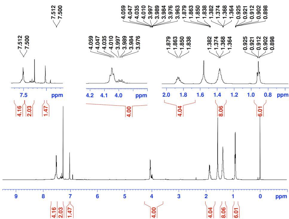
**Fig. S11.**  $^1\text{H}$  NMR spectrum (500 MHz) of poly-**1OH<sub>6</sub>** in  $\text{CDCl}_3$  at 25 °C.
