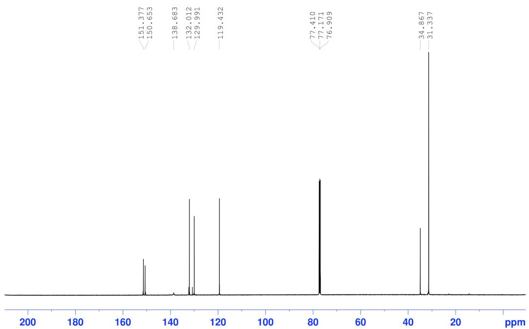
**Fig. S8.**  $^{13}\text{C}$  NMR spectrum (125 MHz) of **1<sub>tBu</sub>** in  $\text{CDCl}_3$  at 25 °C.
