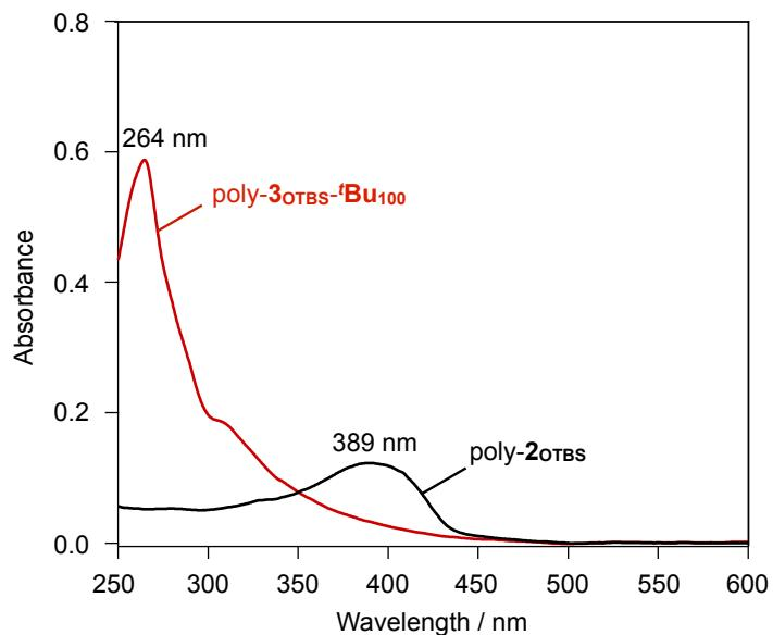
**Fig. S1.** Electronic absorption spectra of poly-**2OTBS** (black,  $3.2 \times 10^{-3}$  mg mL $^{-1}$ ) and poly-**3OTBS-<sup>t</sup>Bu<sub>100</sub>** (red,  $3.2 \times 10^{-3}$  mg mL $^{-1}$ ) in CH<sub>2</sub>Cl<sub>2</sub> at 25 °C.
