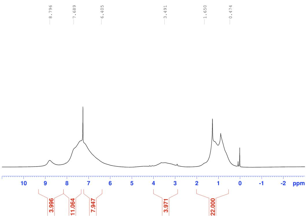
**Fig. S20.** <sup>1</sup>H NMR spectrum (500 MHz) of poly-3OHex-H<sub>100</sub> in CDCl<sub>3</sub> at 25 °C.
