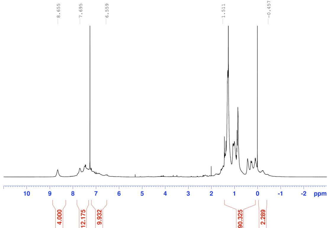
**Fig. S15.**  $^1\text{H}$  NMR spectrum (500 MHz) of poly-3OTBS- $t\text{Bu}_{50}$  in  $\text{CDCl}_3$  at 25 °C.
