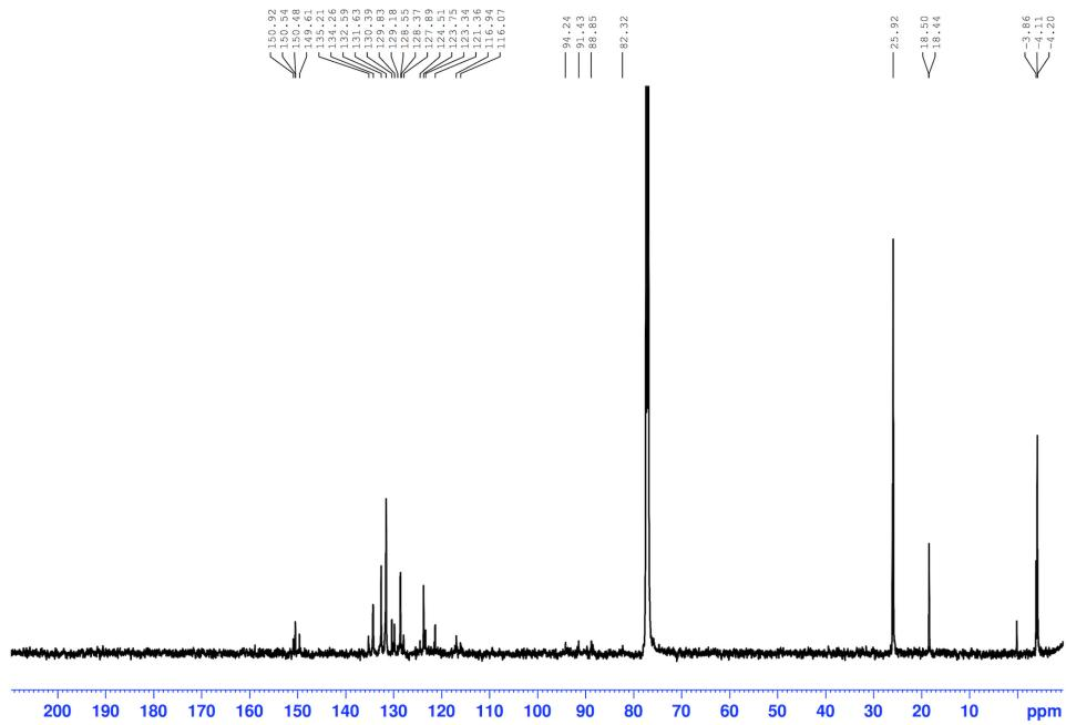
**Fig. S10.**  $^{13}\text{C}$  NMR spectrum (125 MHz) of poly-**1**<sub>0hex</sub> in  $\text{CDCl}_3$  at 25 °C.
