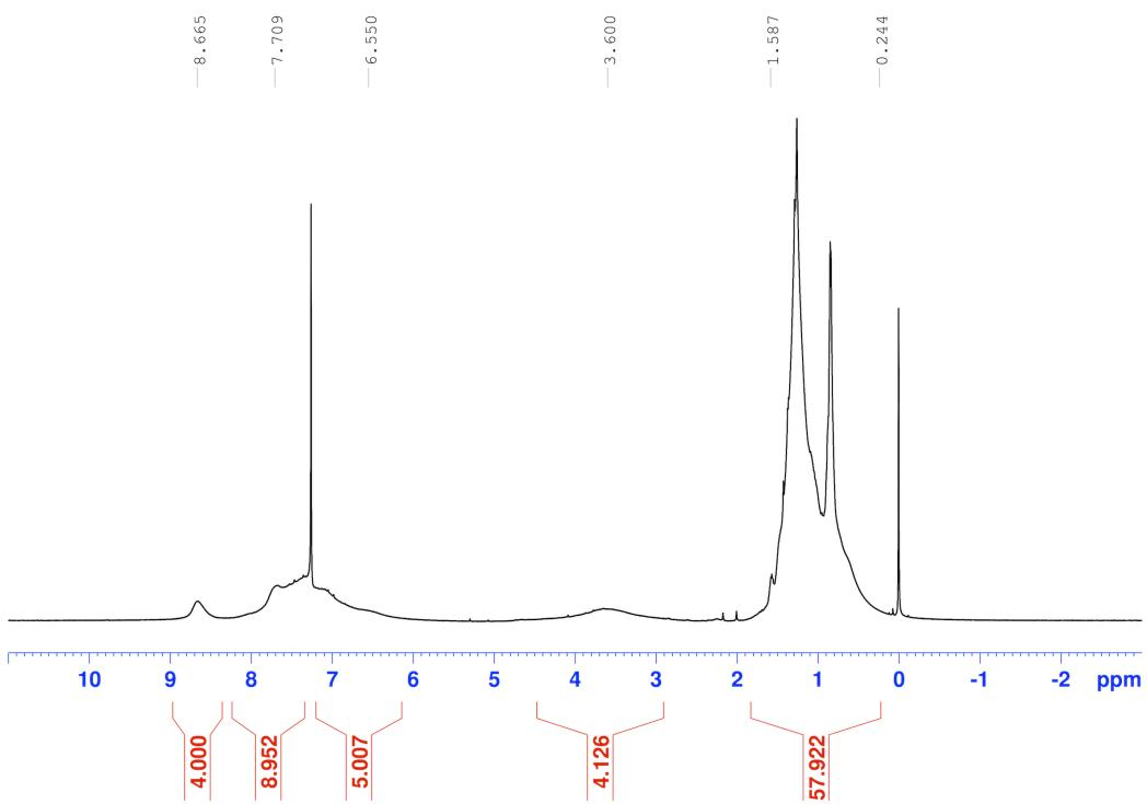
**Fig. S18.** <sup>1</sup>H NMR spectrum (500 MHz) of poly-3OHex-<sup>t</sup>Bu<sub>100</sub> in CDCl<sub>3</sub> at 25 °C.
