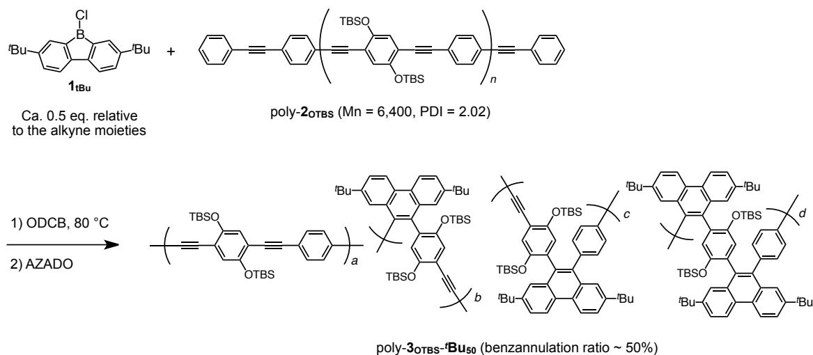
**Scheme S1.** Synthesis of poly-**3**<sub>OTBS-tBu50</sub> from poly-**2**<sub>OTBS</sub>. Possible partial structures of poly-**3**<sub>OTBS-tBu50</sub> are shown.
