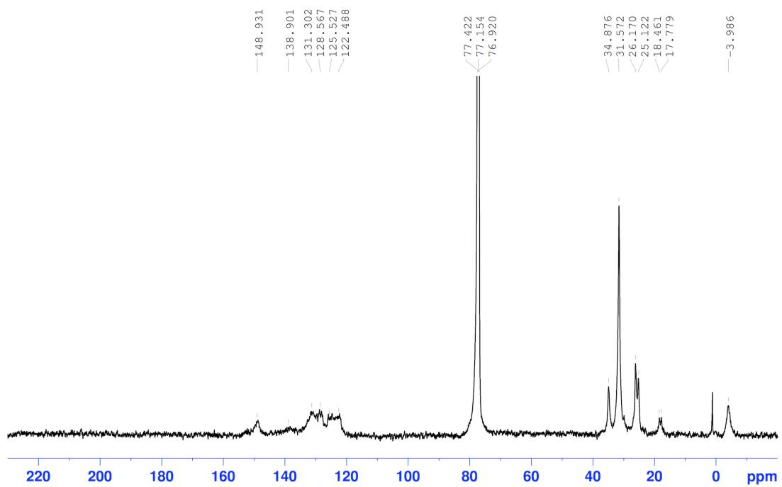
**Fig. S14.**  $^{13}\text{C}$  NMR spectrum (125 MHz) of poly-3OTBS- $t\text{Bu}_{100}$  in  $\text{CDCl}_3$  at 25 °C.
