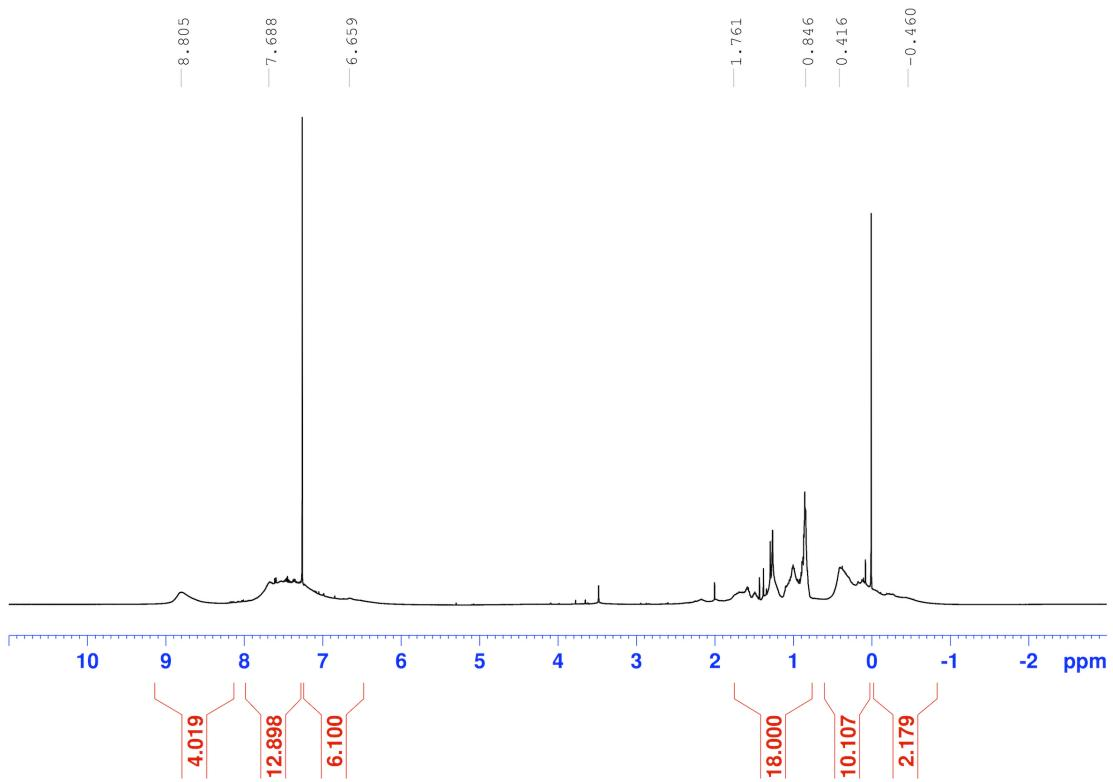
**Fig. S17.**  $^1\text{H}$  NMR spectrum (500 MHz) of poly-3OTBS-H<sub>100</sub> in  $\text{CDCl}_3$  at 25 °C.
