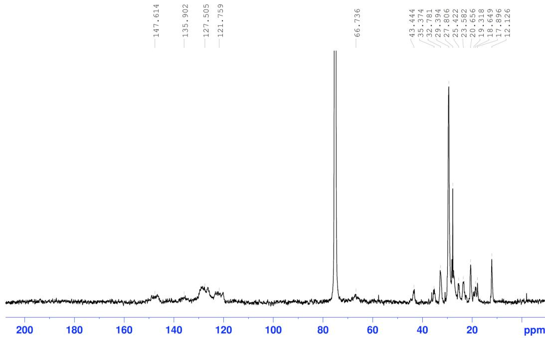
**Fig. S19.** <sup>13</sup>C NMR spectrum (125 MHz) of poly-3OHex-<sup>t</sup>Bu<sub>100</sub> in CDCl<sub>3</sub> at 25 °C.
