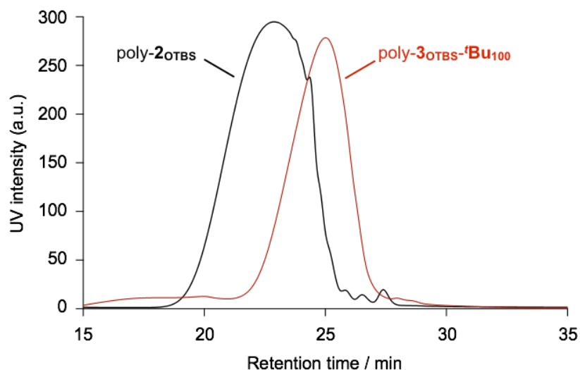
**Fig. S2.** GPC profiles of poly-**2OTBS** ( $M_n = 6,400$  Da, PDI = 2.02) and poly-**3OTBS-<sup>t</sup>Bu<sub>100</sub>** (eluent: CHCl<sub>3</sub>).
