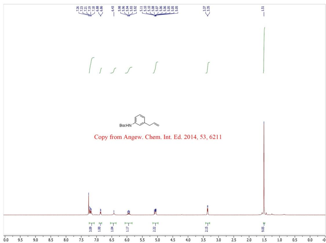
**Fig. S37.**  $^1\text{H}$  NMR (400 MHz,  $\text{CDCl}_3$ )  $\delta$  7.25-7.15 (m, 3H), 6.88 (d,  $J = 7.2$  Hz, 1H), 6.44 (s, 1H),
