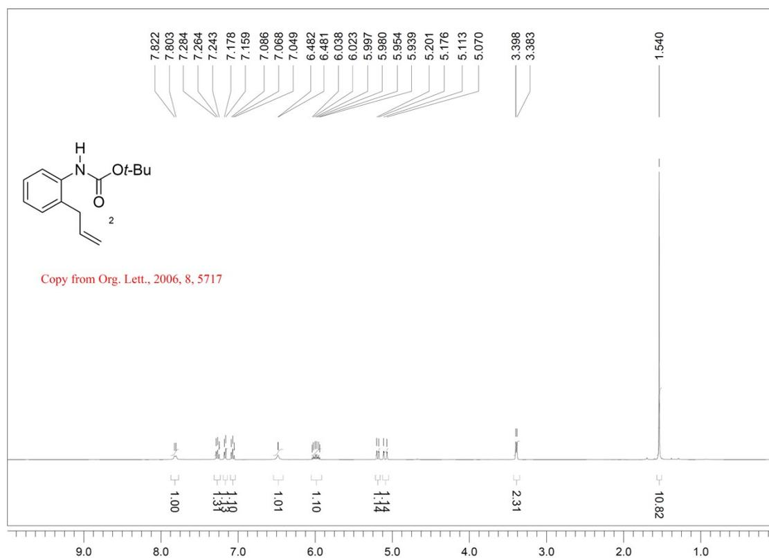
**Fig. S38.**  $^1\text{H}$  NMR (400 MHz,  $\text{CDCl}_3$ )  $\delta$  7.81 (d,  $J = 7$  Hz, 1H), 7.26 (t,  $J = 8$  Hz, 1H), 7.17 (d,  $J = 7$  Hz, 1H), 7.07 (t,  $J = 7$  Hz, 1H), 6.48 (s (br), 1H), 5.99 (ddt,  $J = 17, 10, 6$  Hz, 1H), 5.20-5.17 (m, 1H), 5.11-5.07 (m, 1H), 3.39 (d,  $J = 6$  Hz, 2H), 1.54 (s, 9H).
