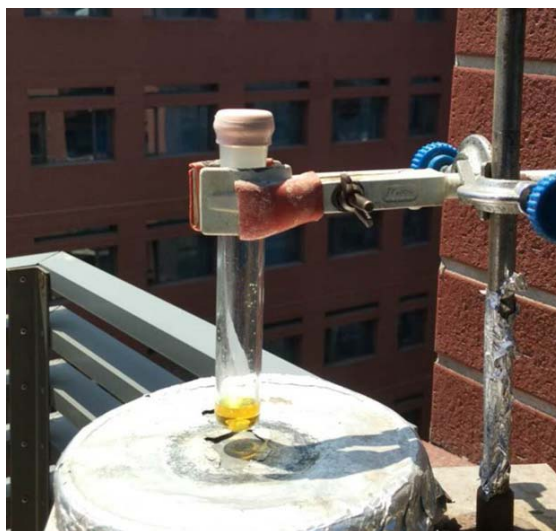
Figure S2. The reaction set-up under sunlight irradiation.
