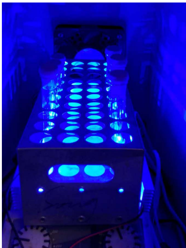
Figure S1. The reaction set-up (commercially available 3 W blue LEDs).
