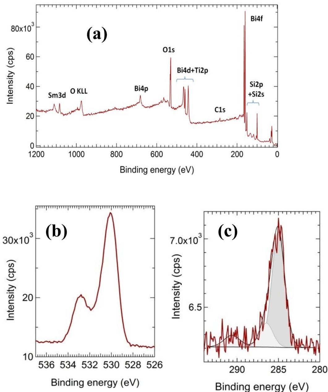
The O 1s region shows a main feature centered at 530.1 eV (fig. S2 b), assigned to the oxide from the SBVT compound. The smaller component at higher BE (fig. S2 c) is attributed to oxygen atoms in SiO<sub>2</sub>, the native oxide on Si wafers, and adsorbed surface species, such as hydroxyl groups and CO like species.
