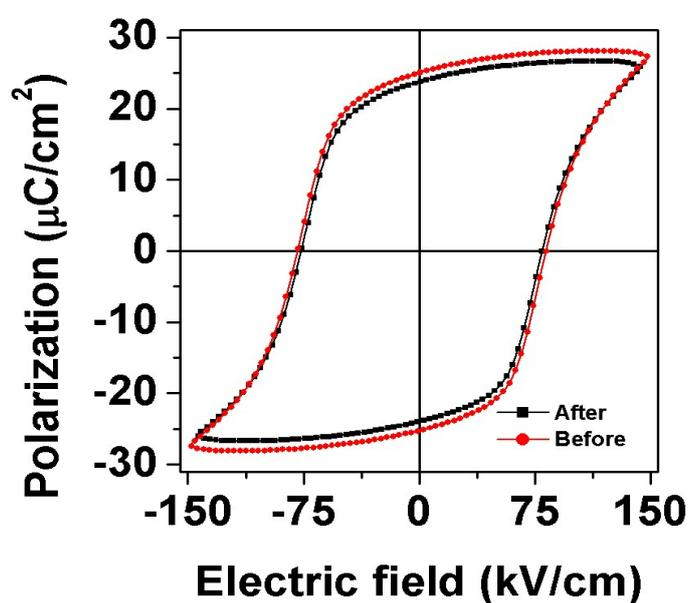
Polarization – electric field hysteresis loops measured before and after 10<sup>8</sup> switching cycles.
