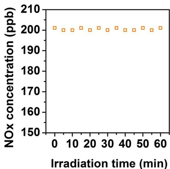
As it is shown in fig. S1, the effect of photolysis to the photocatalytic activity, after 60 min irradiation time, is negligible.
