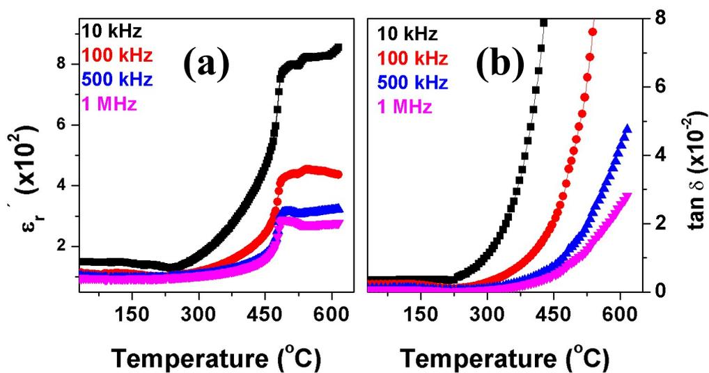
Temperature dependent dielectric constant ( $\epsilon_r'$ ) and  $\tan \delta$  measured at 10 kHz, 100 kHz, 500 kHz and 1 MHz. The arrow in  $\tan \delta$  indicates the phase transition temperature.
