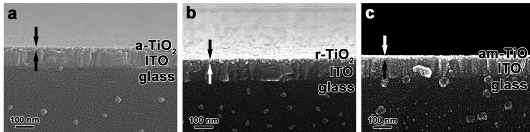
**Fig. S1** The cross-sectional SEM images different kinds of TiO<sub>2</sub> layer on ITO glass. a. anatase TiO<sub>2</sub> layer; b. rutile TiO<sub>2</sub> layer; c. amorphous TiO<sub>2</sub>. The thicknesses of these three kinds of TiO<sub>2</sub> layers are around 25 nm.
