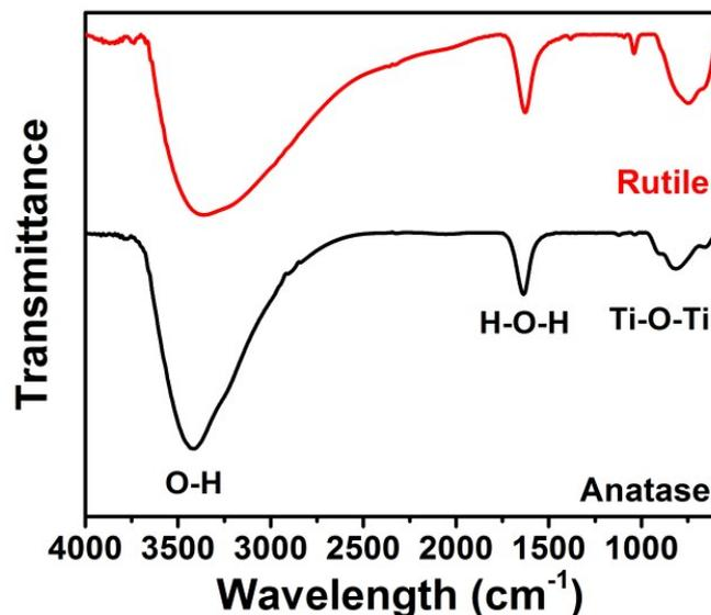
**Fig. S2** The FTIR spectra of anatase and rutile TiO<sub>2</sub> nanocrystals.
