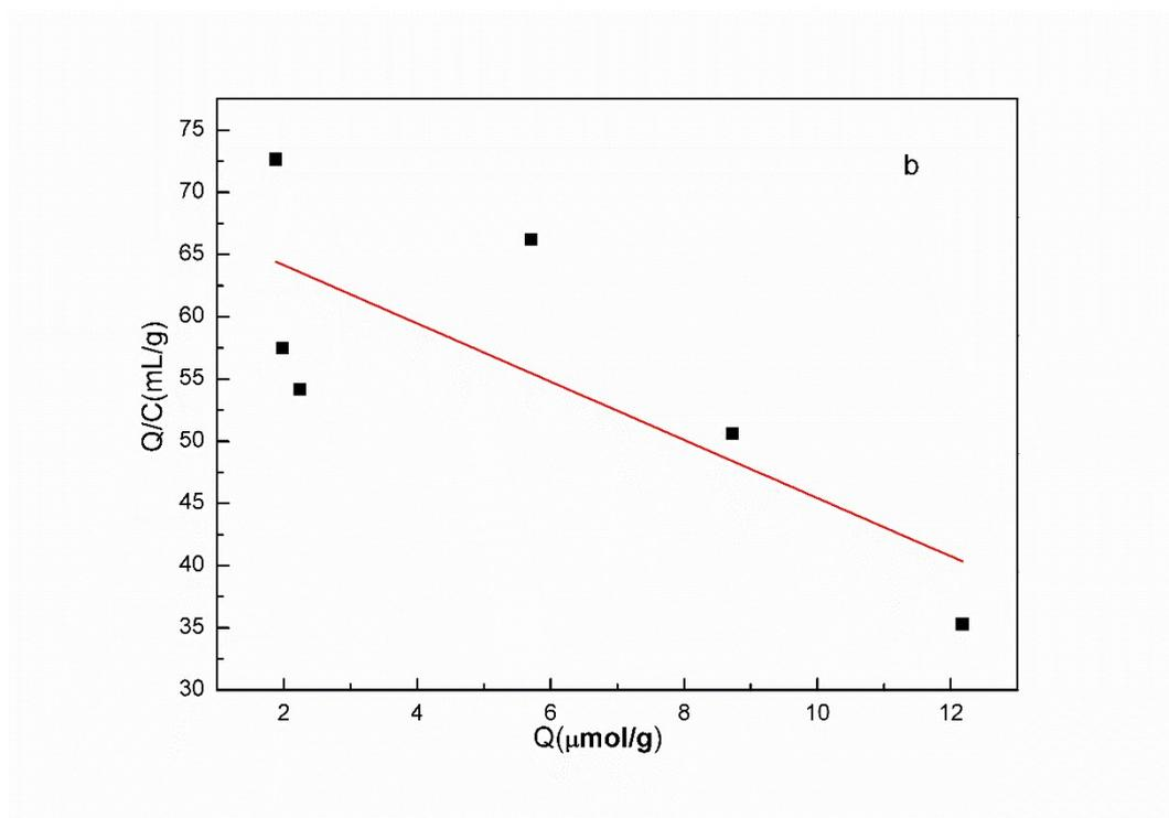
Fig. S5 Scatchard plot analysis of the binding of naringin to SMIPs (a) and SNIPs (b).
