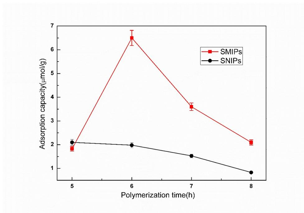
Fig. S3 Effect of polymerization time on the adsorption of naringin onto SMIPs and SNIPs. Initial concentration of naringin=20 mg/L, T=298 K, contact time=5 min.
