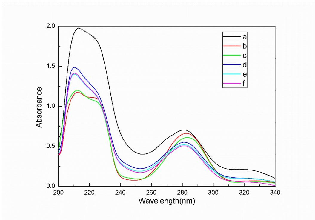
Fig. S7 UV absorption spectra of the grapefruit extract (a), the pure naringin (c), the solution after the first adsorption of SNIPs(b), the solution after adsorption of SMIPs(d, e, f): (f) after the first adsorption; (e) after the second adsorption, (d) after the third adsorption.
