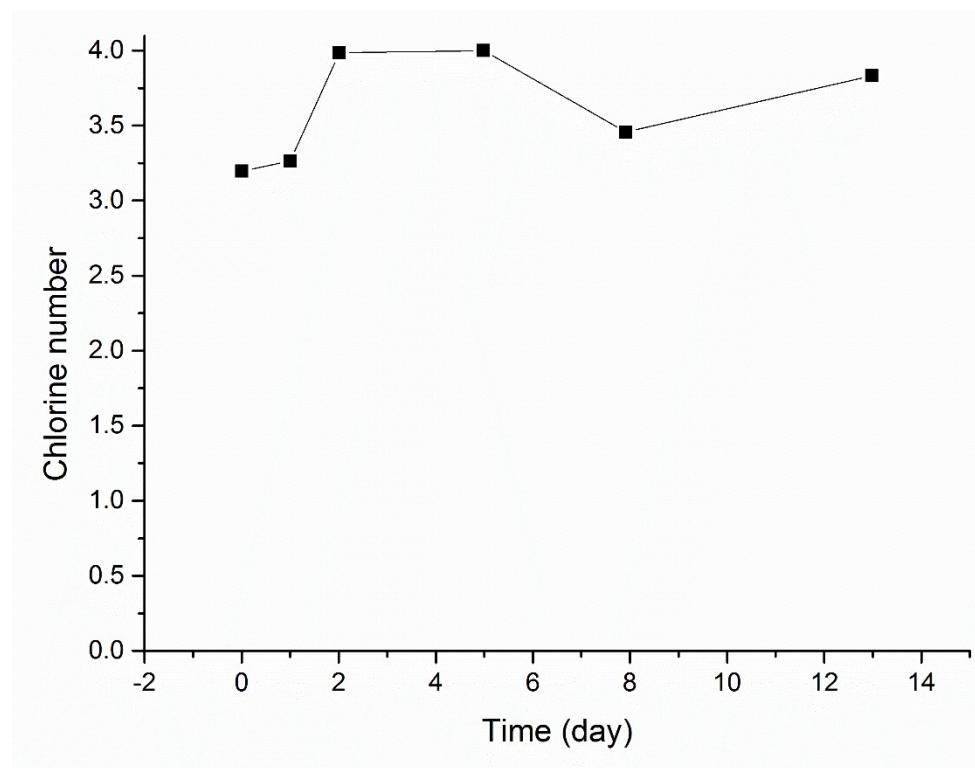
Figure S 1 (supplementary information) : The variation of chlorine number as a function of time during the dechlorination process.
