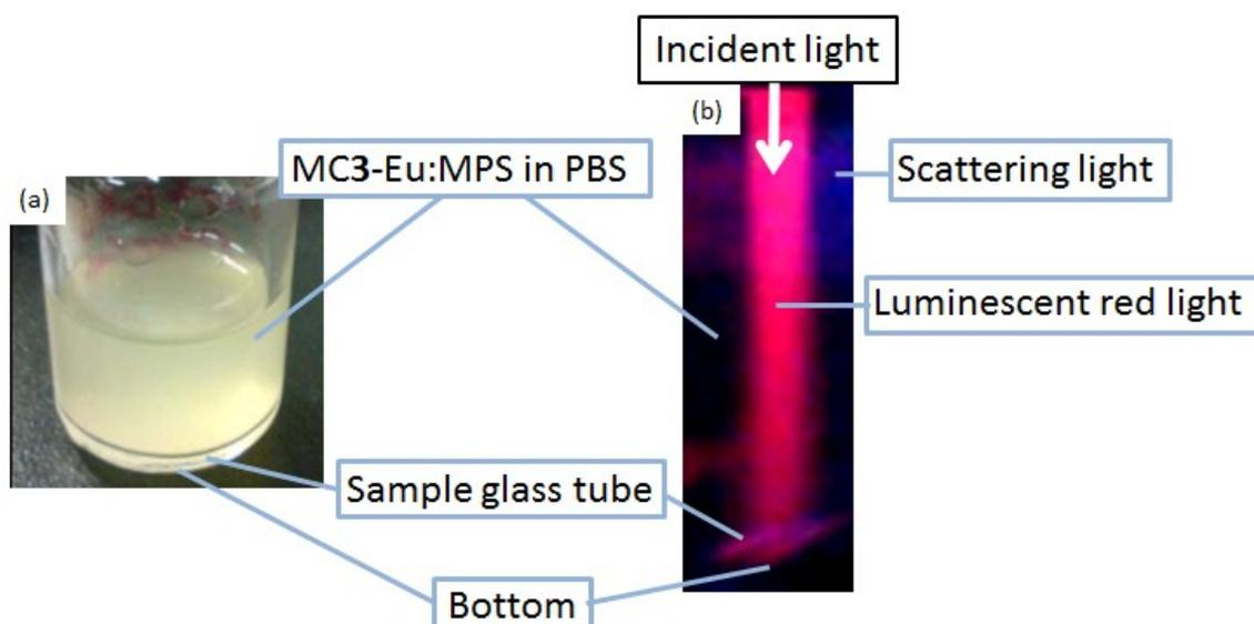
**Fig. S4** Photographs of (a) bright-field and (b) fluorescent images of the MC3-Eu:MPS in PBS at the concentration of 500  $\mu\text{g/mL}$ . The excitation in (b) was conducted using the fluorescent microscope light at the wavelength of 380–420 nm.
