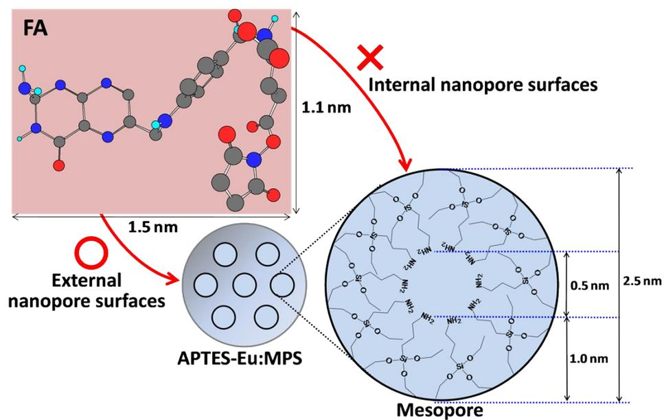
**Scheme S1** Scheme of the FA incorporation into the external and internal nanopore surfaces. The internal nanopore size after the immobilization with monolayer APTES becomes approx. 0.5 nm even if overestimated, indicating the difficulty in the FA incorporation into the nanopore.
