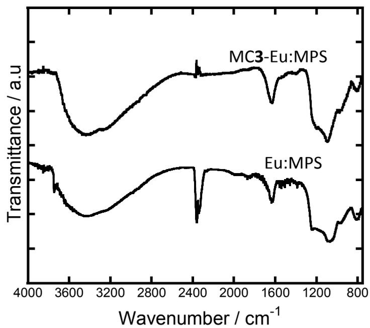
**Fig. S5** FT-IR spectra of the Eu:MPS and MC3-Eu:MPS particles.
