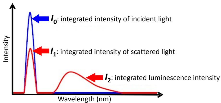
**Scheme S2** Scheme of the representative incident, scattering, and luminescence light intensity spectra for the calculation of internal quantum efficiency. The integrated peak intensities attributed to the incident, scattering, and luminescence were abbreviated as  $I_0$ ,  $I_1$  and  $I_2$ , respectively.
