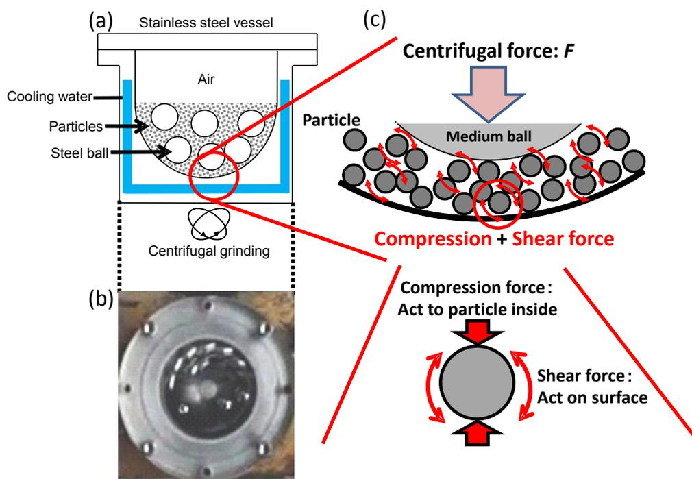
**Fig. S1** (a) Scheme of the set-up for the mechanochemical reaction of the Eu:MPS particles and (b) the photograph of the equipment top view during the milling. (c): Possible forces being generated between medium balls and Eu:MPS particles during the milling.
