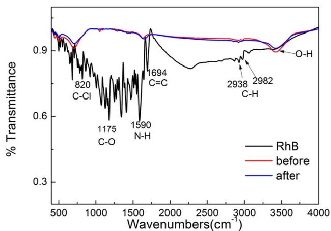
Figure S4. FTIR results of C2 before and after photocatalytic process.
