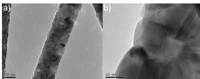
Figure S1. a) TEM and b) HRTEM images of pure TiO<sub>2</sub> nanofibers.
