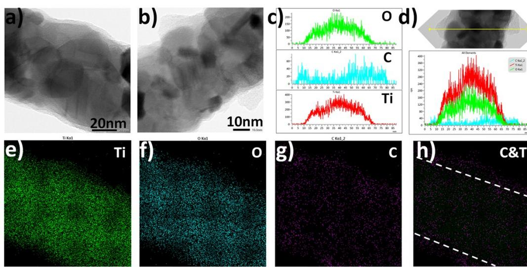
Figure S2. EDS results. a, b) STEM images of C2 and C3. c, d) line scanning results for Ti, O, and Ti of C3. e, f, g, h) mapping results for Ti, O, and C of C2.
