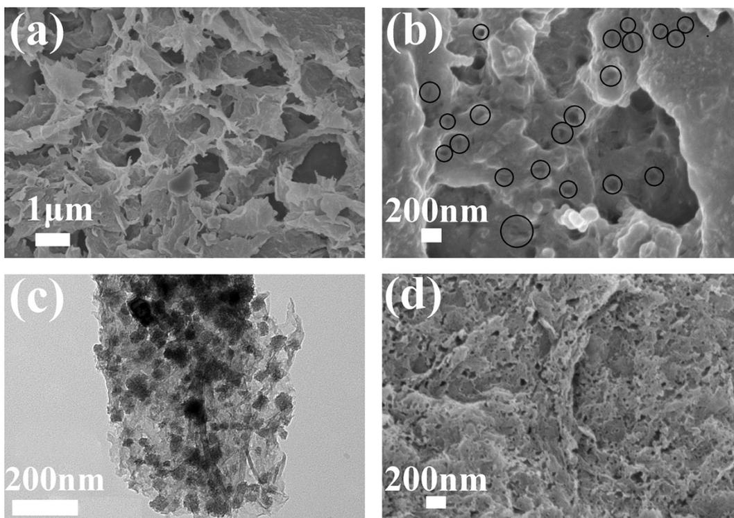
**Figure S4** (a, b) Typical SEM images with different magnifications of MnO/PGA hybrid after 50 cycles at 0.5 A/g. (c) TEM image of MnO/PGA composite after 50 cycles at 0.5 A/g. (d) SEM image of MnO/PGA composite washed with HCl after 50 cycles at 0.5 A/g.
