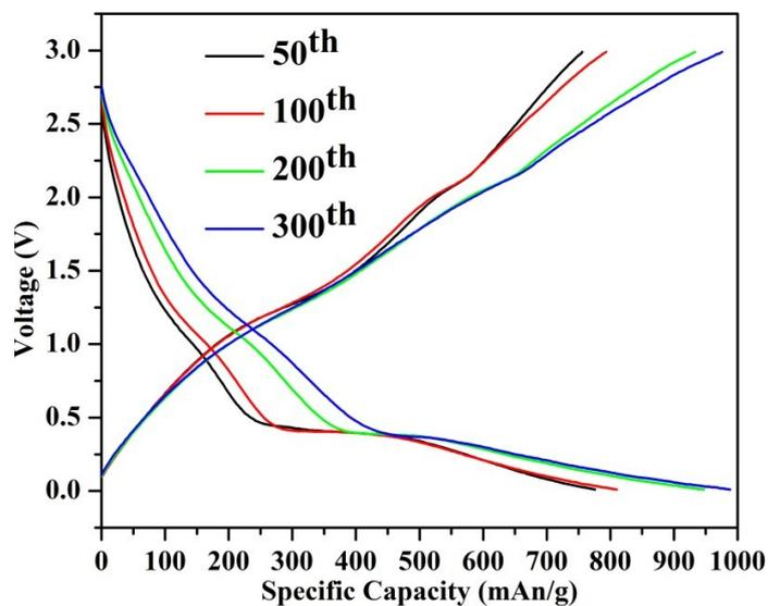
**Figure S3.** The typical charge-discharge curves at the 50<sup>th</sup>, 100<sup>th</sup>, 200<sup>th</sup> and 300<sup>th</sup> cycle during long-term cycles for MnO/PGA at 0.5 A/g.
