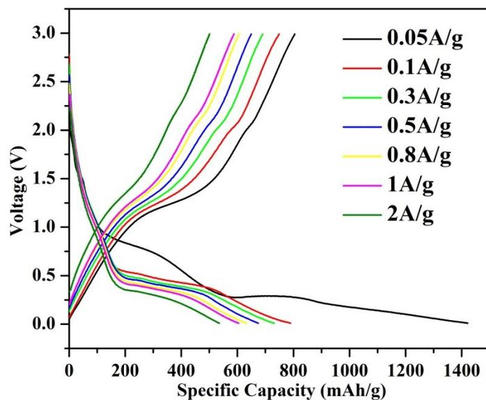
**Figure S2.** The charge-discharge curves of MnO/PGA sample at various current densities of 0.05 A/g, 0.1 A/g, 0.3 A/g, 0.5 A/g, 0.8 A/g, 1 A/g and 2 A/g.
