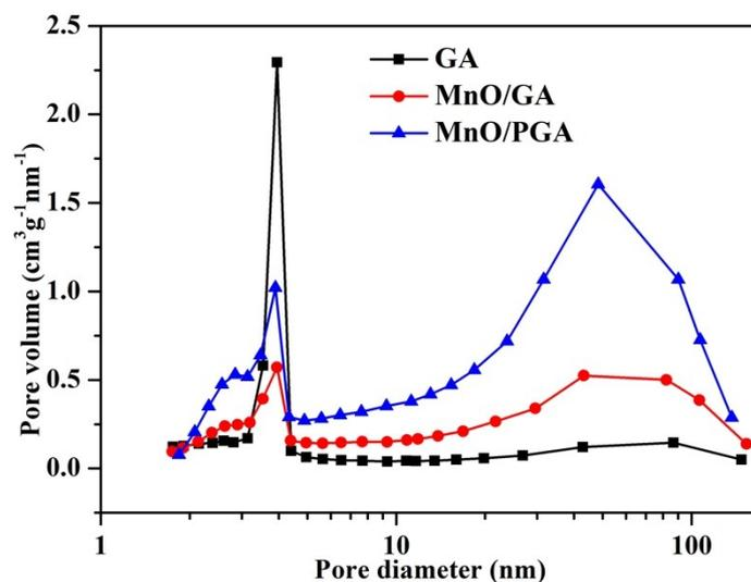
**Figure S1.** Pore size distribution curves of GA, MnO/GA and MnO/PGA samples.
