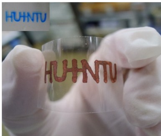
Figure S8. Photograph of a pen-writing copper thin film on PET. The inset picture shows the pattern before calcination.
