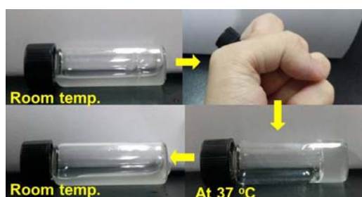
Fig. S9. Vial inversion tests provide visual evidence that the B1 solution formed a hydrogel when the temperature was higher than the sol–gel transition temperature and formed a solution when the temperature back to the room temperature.
