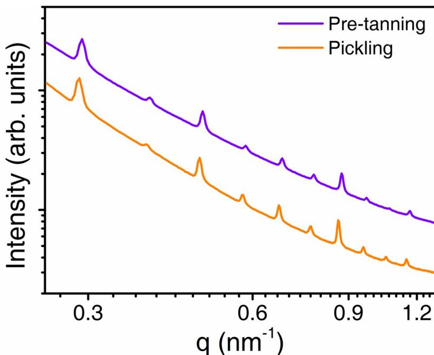
Figure S1: SAXS patterns for pickling stage and pre-tanning stage
