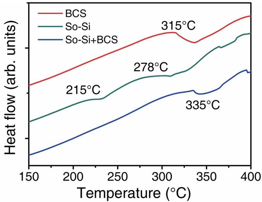
**Figure S2:** DSC plot of dry leather samples. Temperatures indicate the of denaturation of the samples in the dry state.
