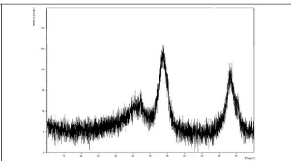
**Figure S2. X-ray diffraction patterns of Mg(Fe)O mixed oxide**
