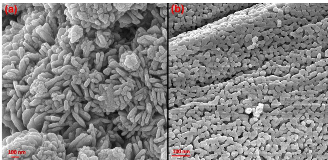
**Fig. S2** (a) FE-SEM image of CuO particles and (b)  $\text{Eu}_2\text{O}_3$  nanoparticles.
