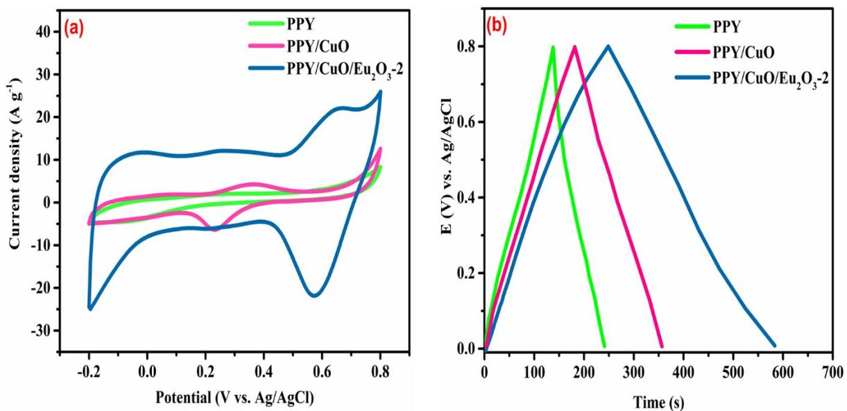
**Fig. S3** The electrochemical performances of PPY, PPY/CuO, and PPY/CuO/Eu<sub>2</sub>O<sub>3</sub> nanocomposites in a three-electrode system (a) CV curves @ 200 mV s<sup>-1</sup> and (b) GCD plots at 1 A g<sup>-1</sup>.
