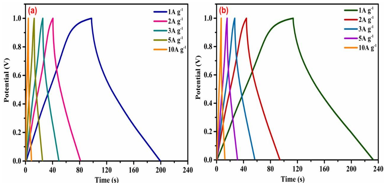
**Fig. S1.** GCD plots of (a) PPY/CuO/Eu<sub>2</sub>O<sub>3</sub>-1 ternary nanocomposite and (b) PPY/CuO/Eu<sub>2</sub>O<sub>3</sub>-3 ternary nanocomposite at the various current densities.
