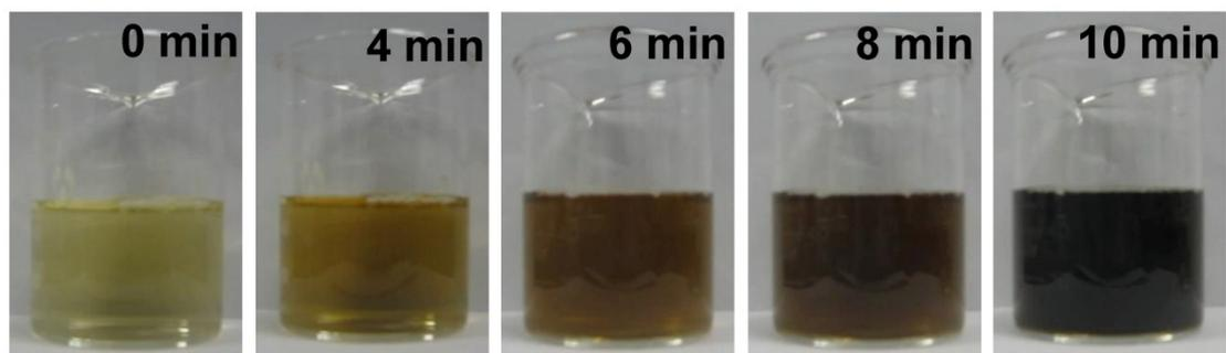
**Fig. S1** Color changes of the reaction solution during the formation process of BSA@Bi<sub>2</sub>S<sub>3</sub> NPs.
