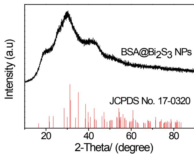
**Fig. S2** XRD pattern of BSA@Bi<sub>2</sub>S<sub>3</sub> NPs.
