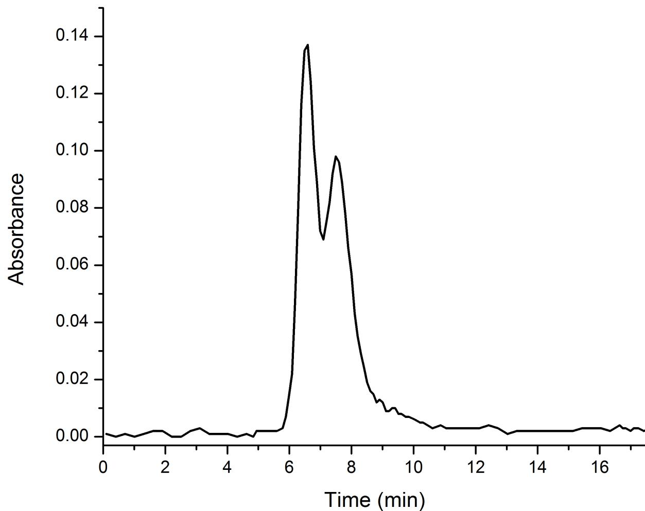
The UV-Vis chromatogram generated by the CombiFlash® Rf+ of a separation of fullerenes using 2-functionalized silica gel and a 25% toluene in hexanes mobile phase. Collected at 380 nm.
