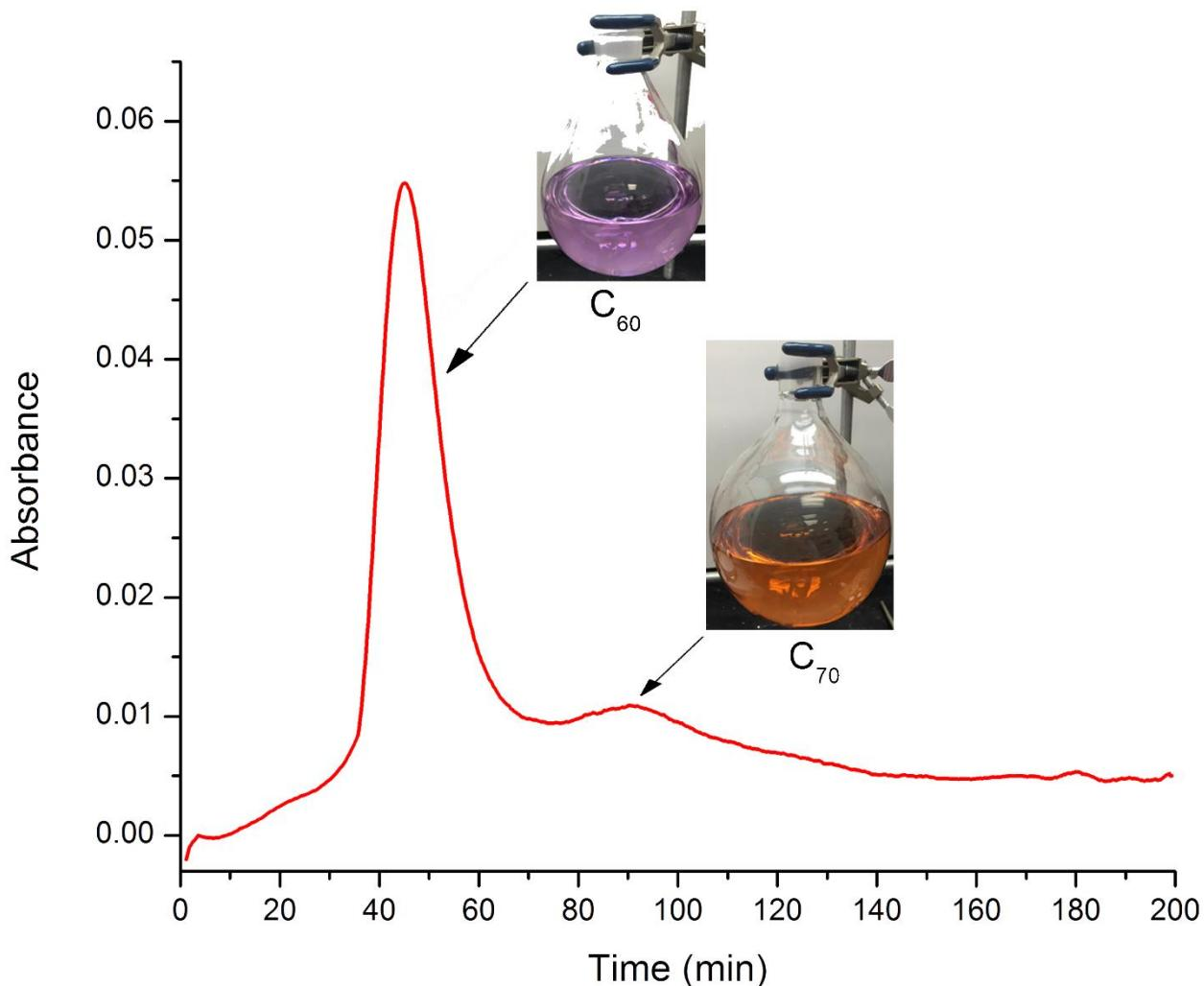
The UV-Vis chromatogram generated by the CombiFlash® Rf+ of a separation of fullerenes using 2-functionalized silica gel and a hexanes mobile phase. Collected at 260 nm. The curve has been smoothed using 30 points of adjacent-averaging. The inset images represent the visual colour of each fraction: pink corresponding to  $C_{60}$  and orange corresponding to  $C_{70}$ .
