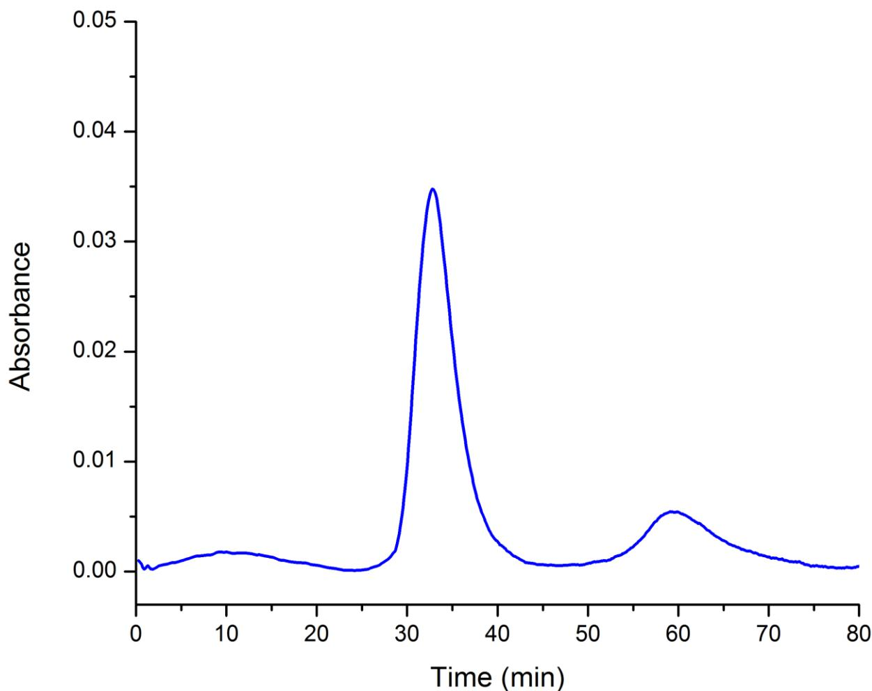
The UV-Vis chromatogram generated by the CombiFlash® Rf+ of a separation of fullerenes using 2-functionalized silica gel and a 25% toluene in hexanes mobile phase. Collected at 290 nm. The curve has been smoothed using 30 points of adjacent-averaging.
