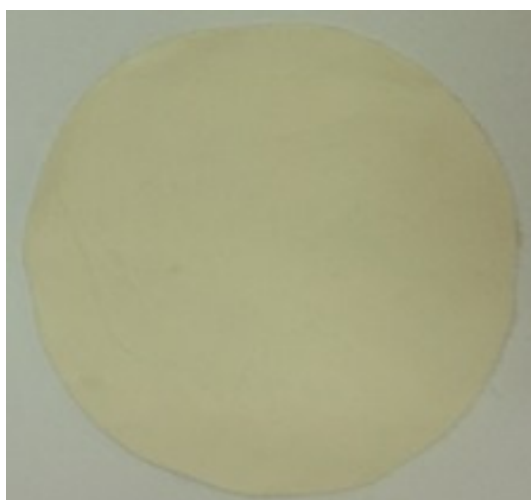
Fig. S6 Photograph of FTPI nanofibrous membrane (membrane diameter: 4cm).
