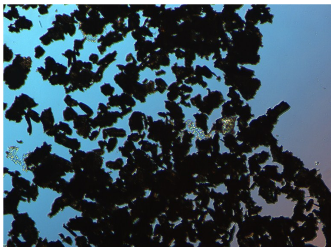
Figure 10: Dissolved and Regenerated cellulose (MCC) from large-scale dissolution experiment (x5 zoom)
