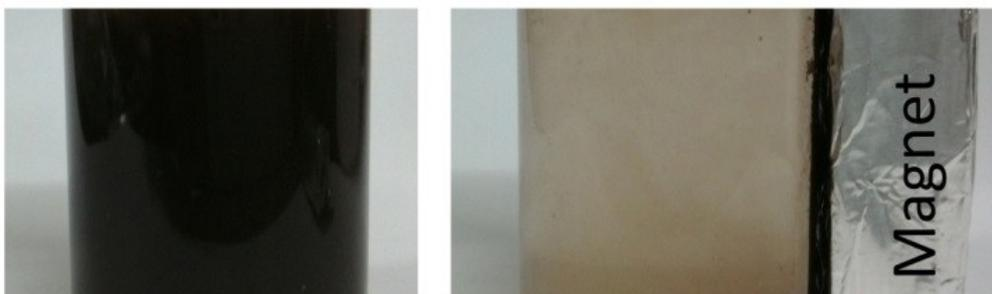
**Fig. S 10 - Separation of ZnFe<sub>2</sub>O<sub>4</sub>-Ag/rGO NC from the suspension using its magnetic property.**
