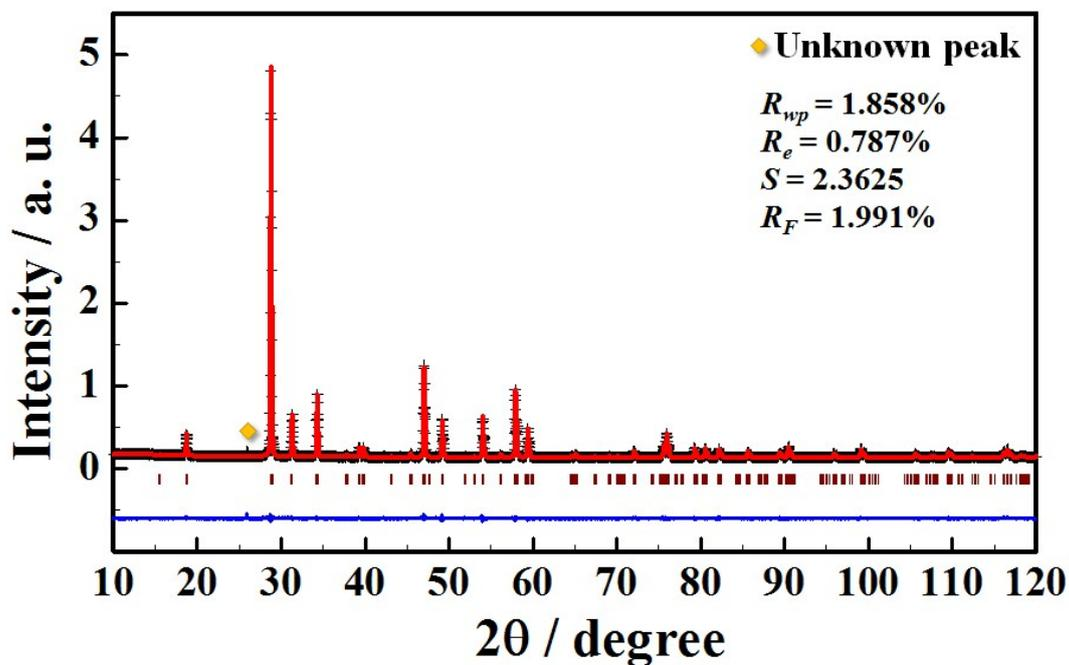
**Figure S1.** Observed (+) and calculated (red line) X-ray powder diffraction data of  $\text{NaEu}(\text{MoO}_4)_2$  phosphor prepared by the conventional SSR method as well as the difference profile (blue bottom line) between them. Bragg reflection peak positions are shown as vertical bars. Inset shows the R-factors and S value of this refinement.
