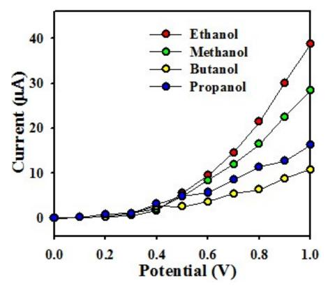
$(\Psi)$  Selectivity of ethanol sensor based on CdO/ZnO/Yb<sub>2</sub>O<sub>3</sub> NSs
