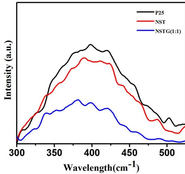
**Fig. S4** PL spectra of P25, NST and NSTG(1:1) under UV-280 nm
