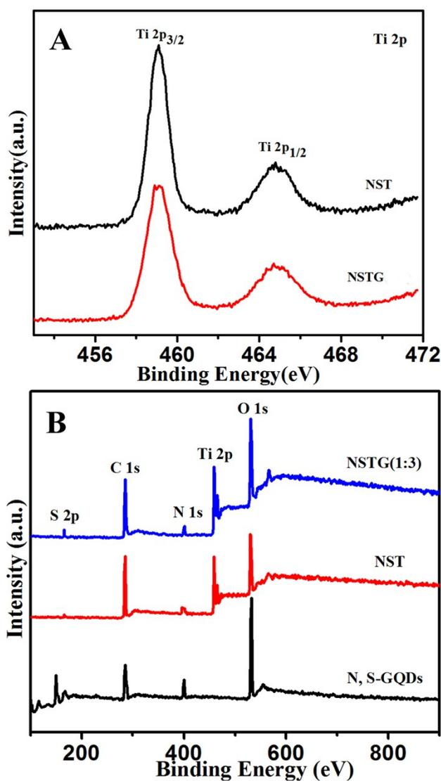
**Fig. S3** (A) High-resolution XPS of Ti 2p for NST and NSTG and (B) XPS full survey spectra of N, S-GQDs, NST and NSTG(1:3)
