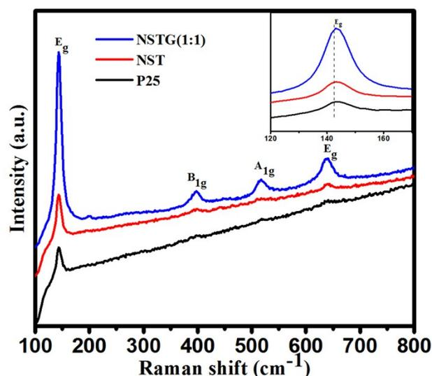
**Fig. S1** Raman spectra of P25, NST and NSTG(1:1). Inset Raman spectra showing the blue shift of the E<sub>g</sub> bands of the composites in the 120-170 cm<sup>-1</sup>.
