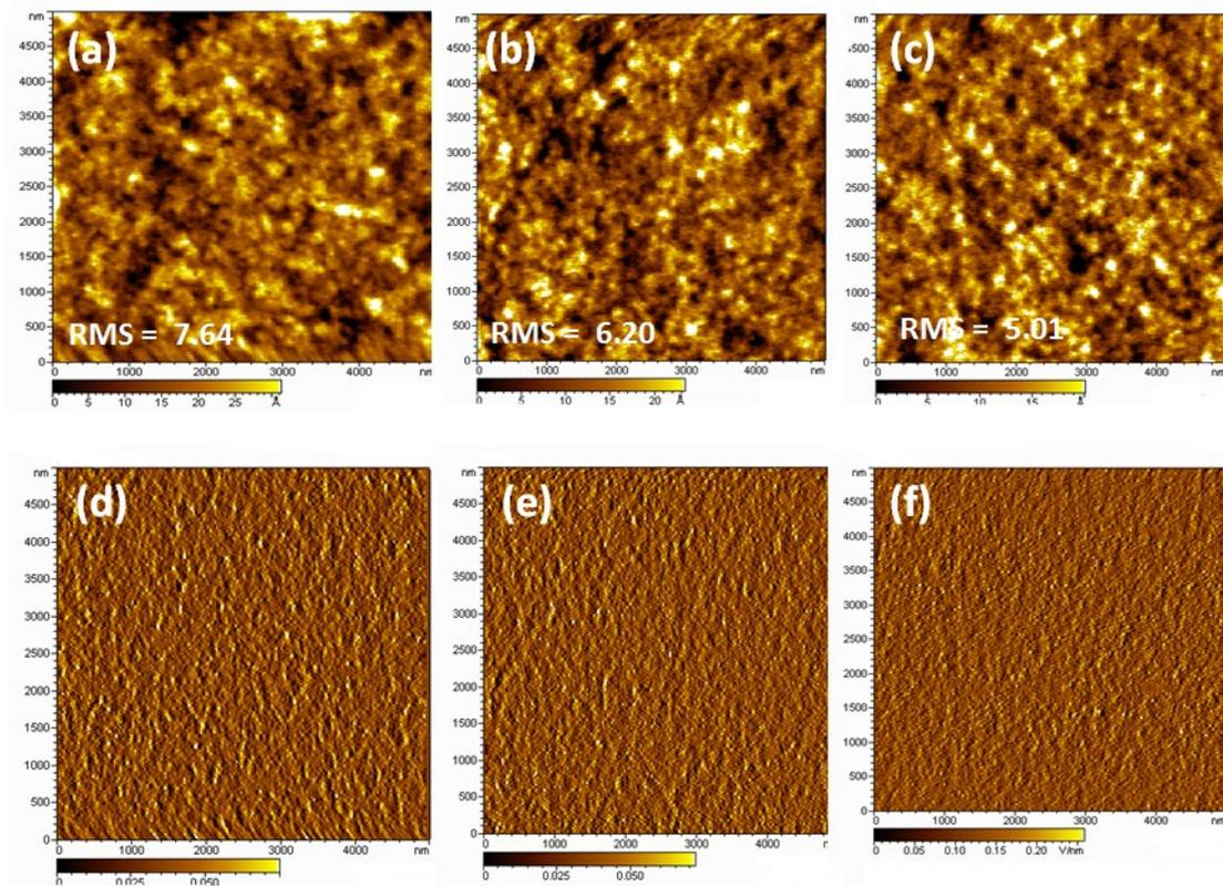
**Fig. S14** AFM images of different D/A blend films: (a, d) (TPACN)<sub>2</sub>Qx:PC<sub>61</sub>BM (1:1, w/w); (b, e) (TPACN)<sub>2</sub>Qx:PC<sub>61</sub>BM (1:3, w/w); (c, f) (TPACN)<sub>2</sub>Qx:PC<sub>61</sub>BM (1:2, w/w).
