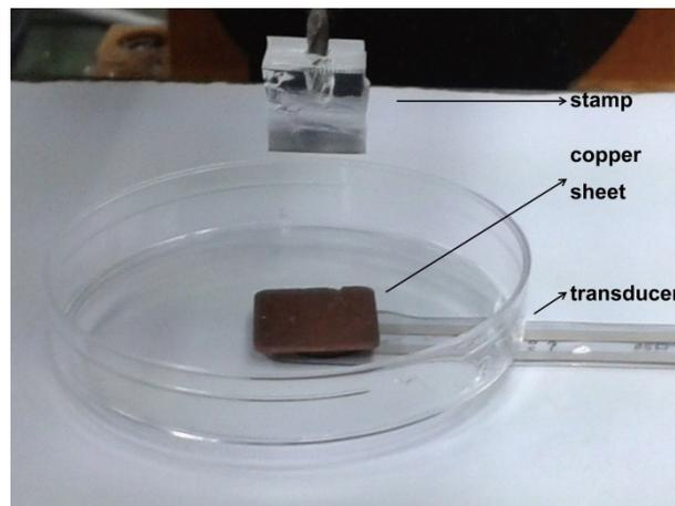
**Fig. S1.** Mechanical transducer setup for measuring minimum pressure applied to induce cell lysis.
