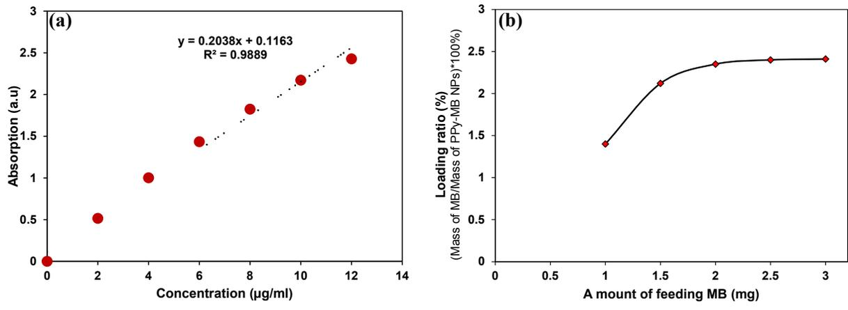
**Figure S1:** (a) The standard curve of MB, and (b) The plot of the loading amount of MB on the PPY NPs.
