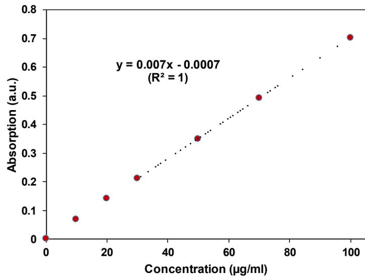
**Figure S2:** The standard curve of PPY-MB NPs (based on 808 nm peak absorption).
