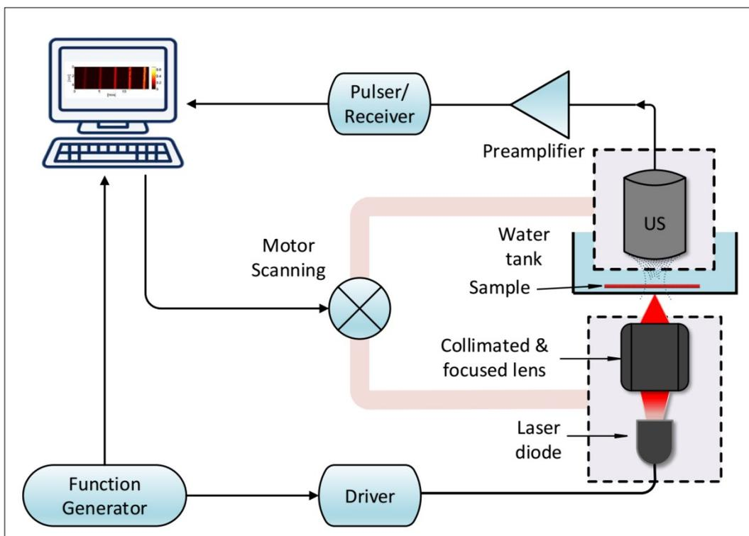
**Figure S10:** Experimental setup of photoacoustic microscopy (PAM) laser diode on PPy-MB NPs injected samples.
