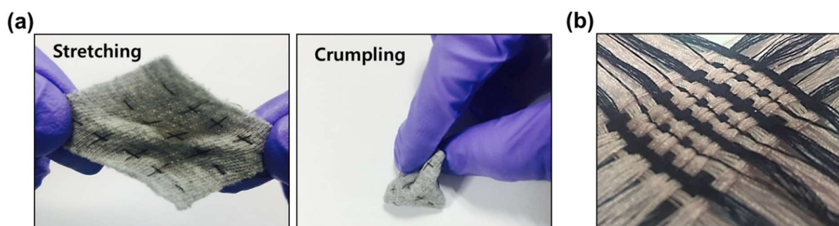
Figure S1. (a) Photographs of i-textile pressure sensor under stretching and crumpling conditions. (b) Wearable woven i-textiles.
