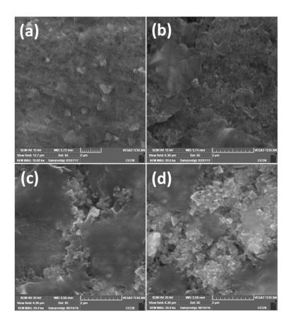
**Figure S1.** Post cycling SEM images of (a-b) ZMO after 150 cycles and (c-d) ZMO/NG nanocomposite electrode after 1000 charge/discharge cycles at a current density of 100 mA g<sup>-1</sup>.
