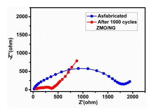
**Figure S3.** Electrochemical impedance spectroscopy of the cell containing ZMO/NG nanocomposite anode recorded for conditions namely as fabricated cell and the cell after completing 1000 cycles
