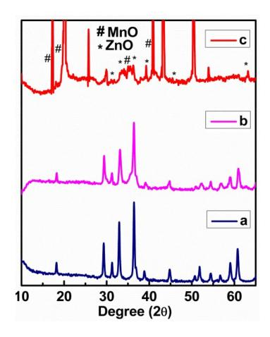
**Figure S2.** XRD pattern of (a) pristine ZMO, (b) ZMO/NG nanocomposite electrode and (c) ZMO/NG nanocomposite electrode after 1000 charge/discharge cycles at a current density of 100 mA g<sup>-1</sup>.
