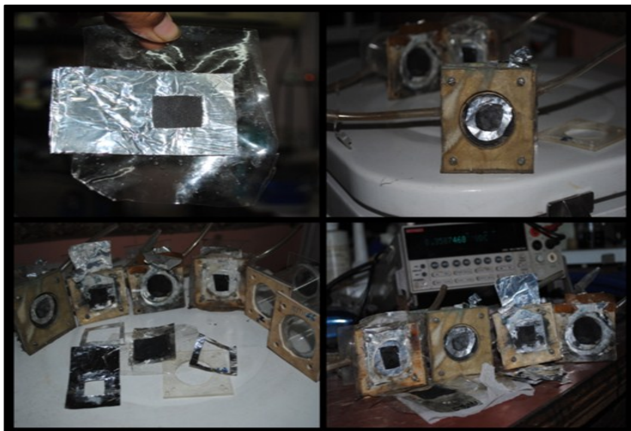
Figure S5: Membrane electrode assembly (MEA) in single chambered MFCs
